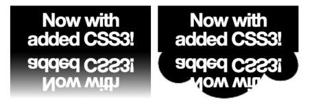
Figure 12-10: Using a gradient (left) and image (right) as a mask
