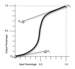
Figure 13-1: An example of a cubic Bézier curve
