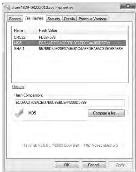
Figure 8-42: The MD5 hashes of the original file and the extracted file are equivalent.
