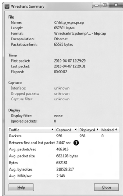
Figure 8-16: The Summary window for the file shows that this entire process occurs in two seconds.
