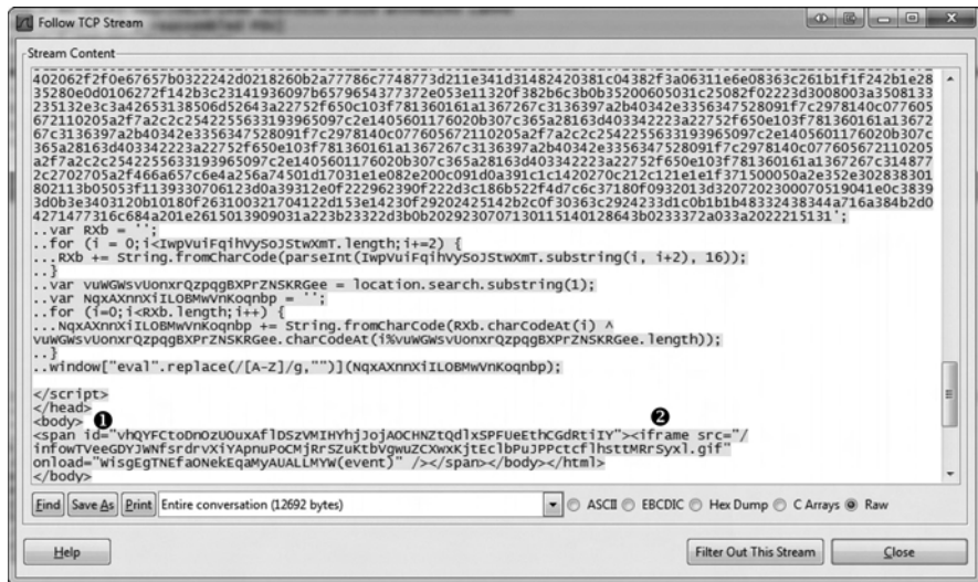
Figure 10-12: This portion of the content sent from the server contains readable text and a suspicious iframe.
