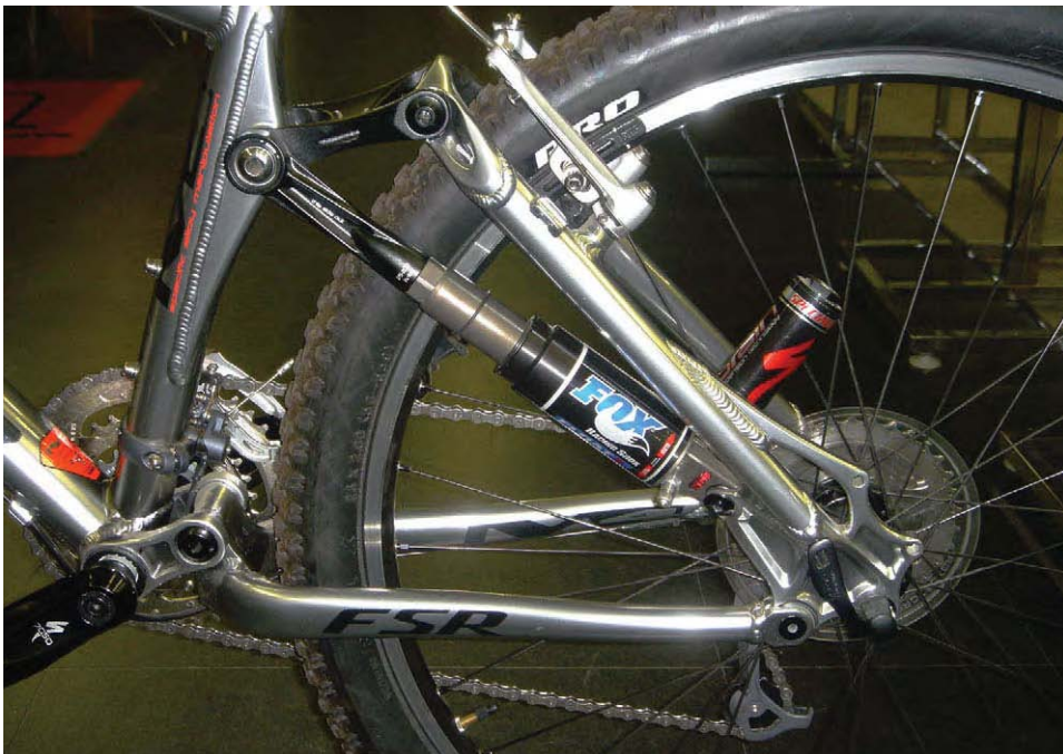
Figure 30: Specialized Epic Bicycle with Inertia Valve Shock
