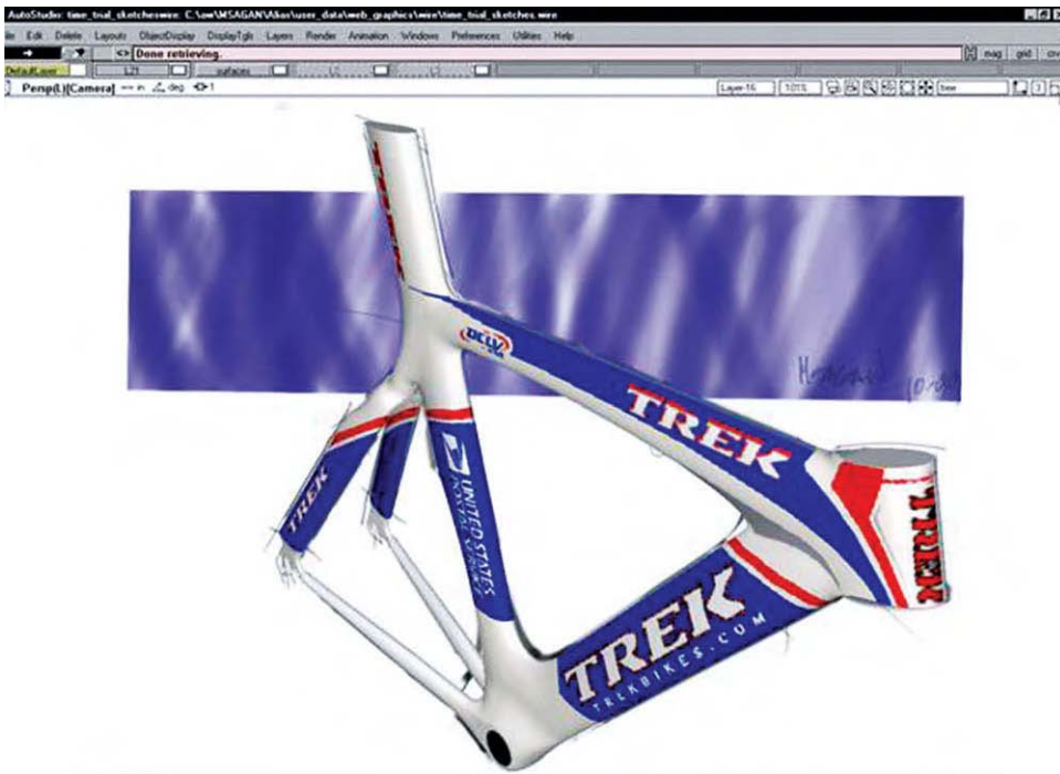
Figure 38: Accurate 3D Shaded Model Superimposed Over Three-Quarter View Sketch
