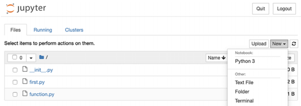
Figure A.16 Selecting the menu option to create a new Python 3 notebook
