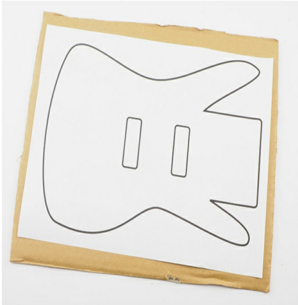
Figure 3-3: Gluing the paper template to the cardboard
