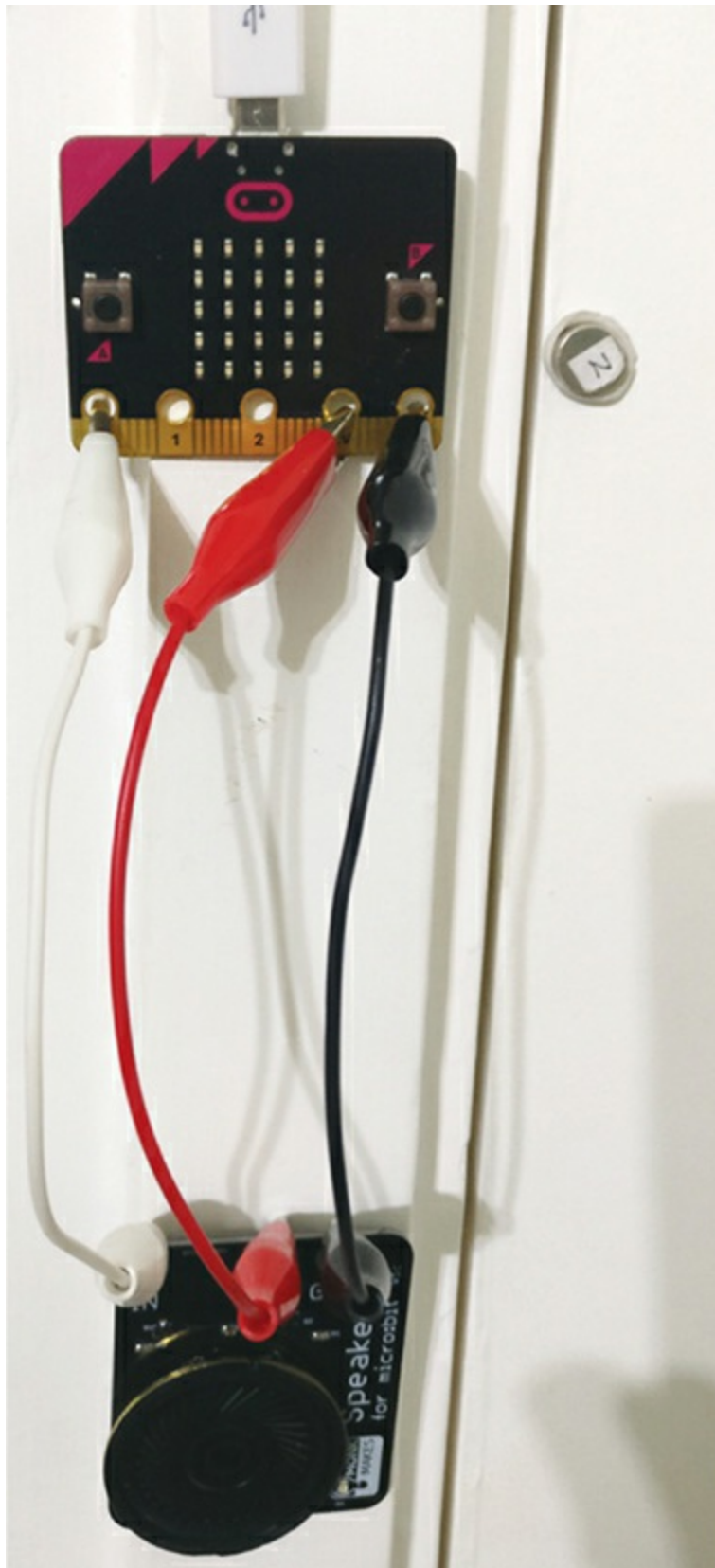
Figure 4-9: A magnetic door alarm
