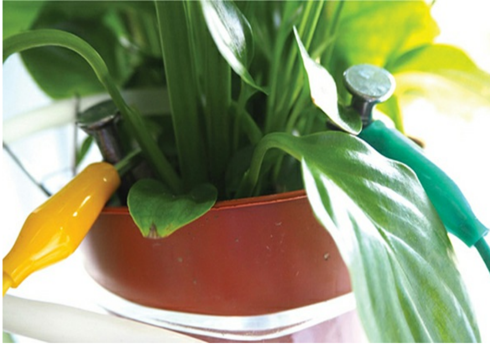
Figure 9-8: Positioning the nails in the soil
