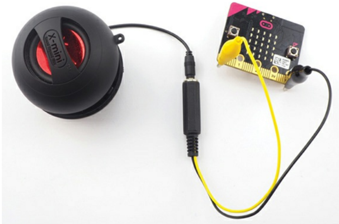
Figure 2-3: Connecting a micro:bit to an amplified speaker
