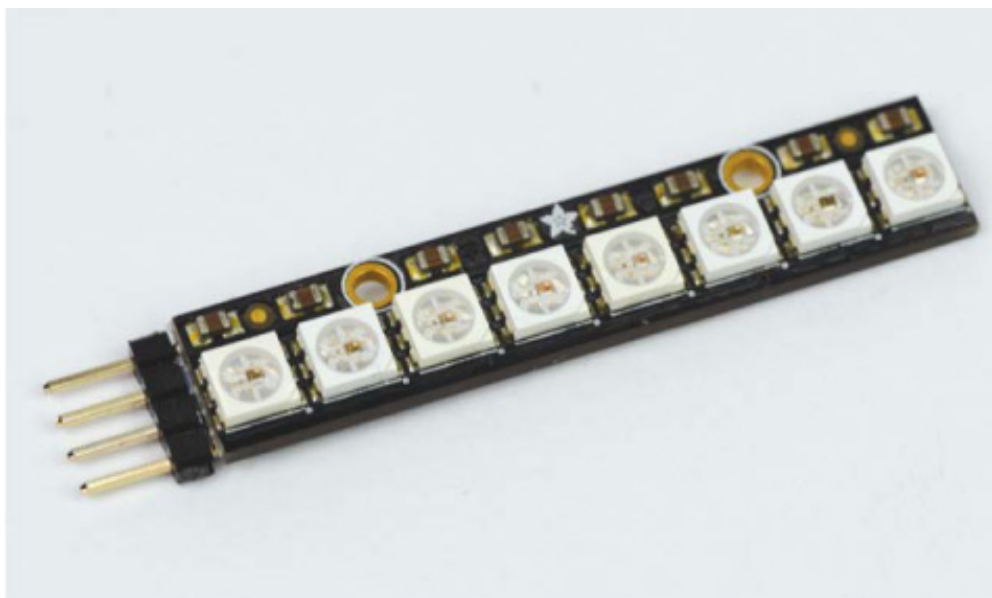
FIGURE 6-4 NeoPixel Stick with headers soldered on
