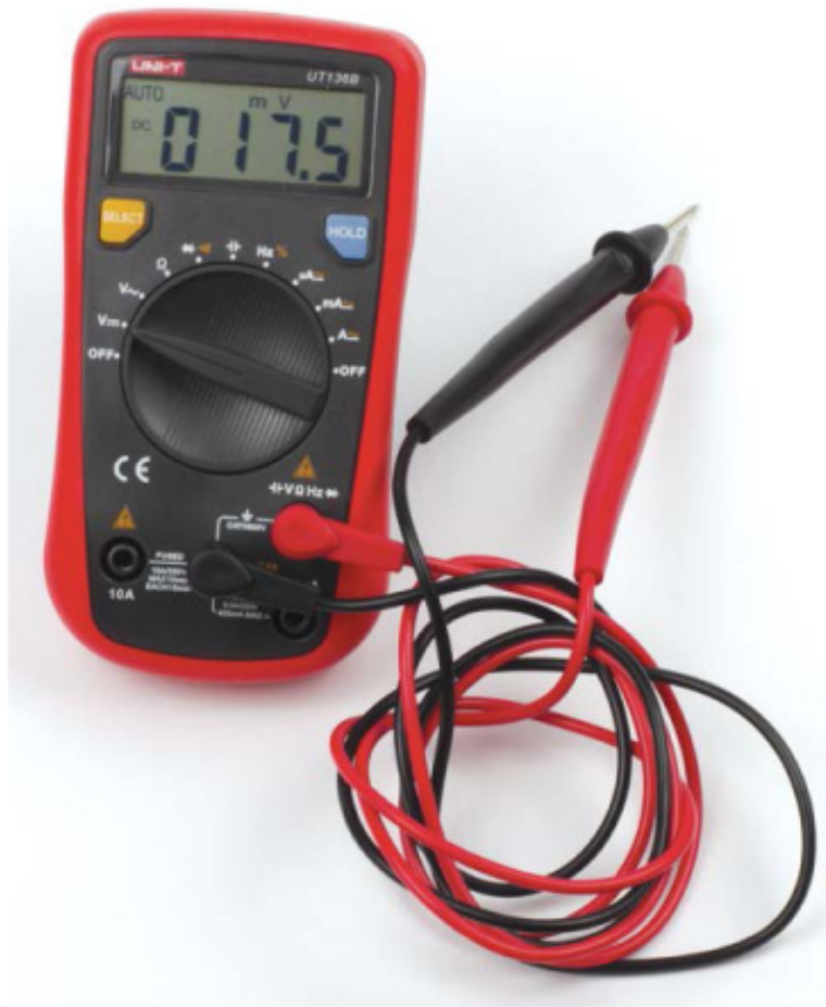
FIGURE 3-17 A multimeter, set to read voltage
