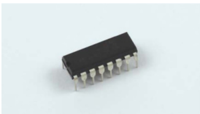
FIGURE 3-9 An L293D motor controller chip
