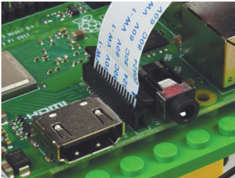
FIGURE 8-5 CSI port with the Camera Module’s ribbon cable inserted in the correct direction
