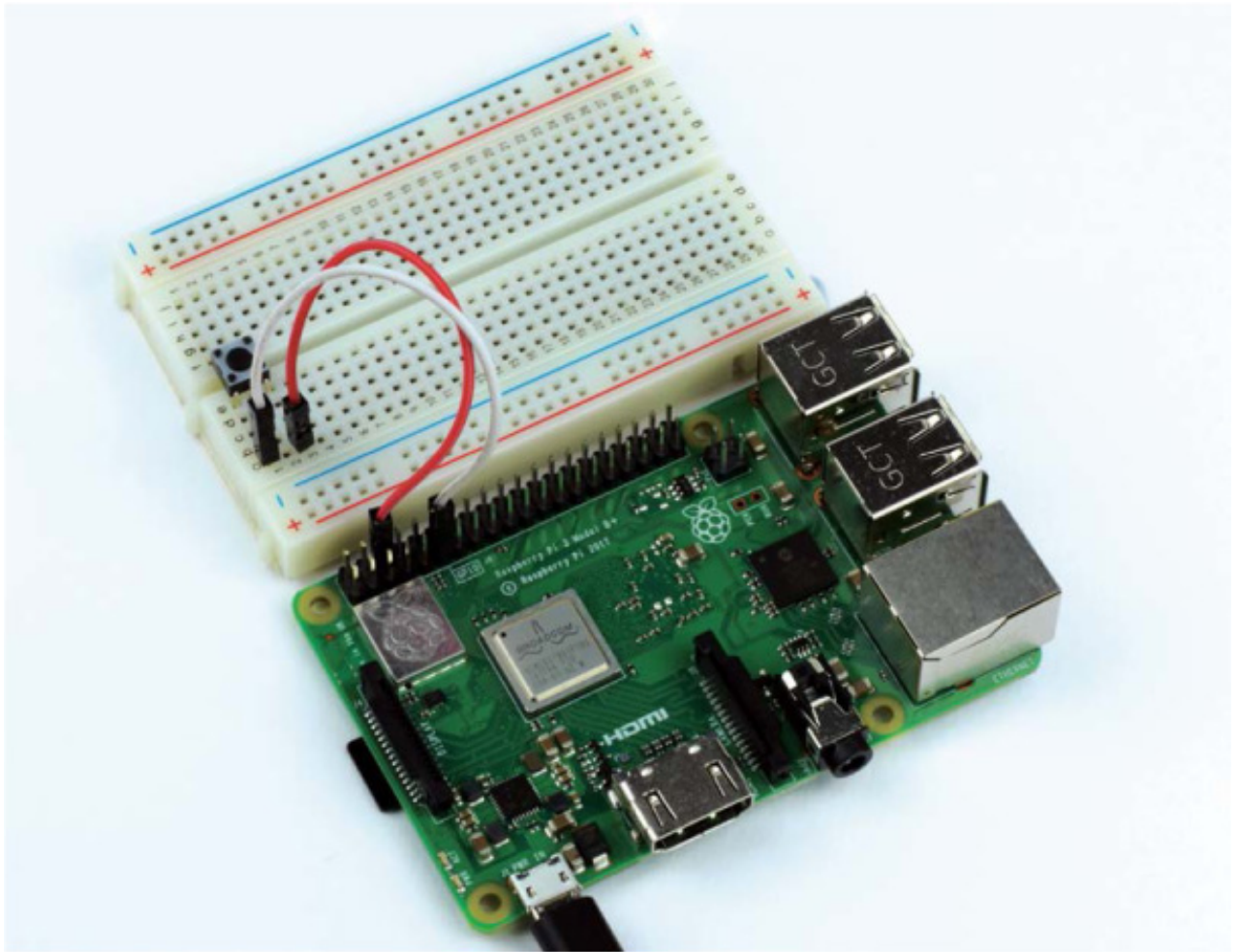
FIGURE 2-12 The complete button and breadboard setup
