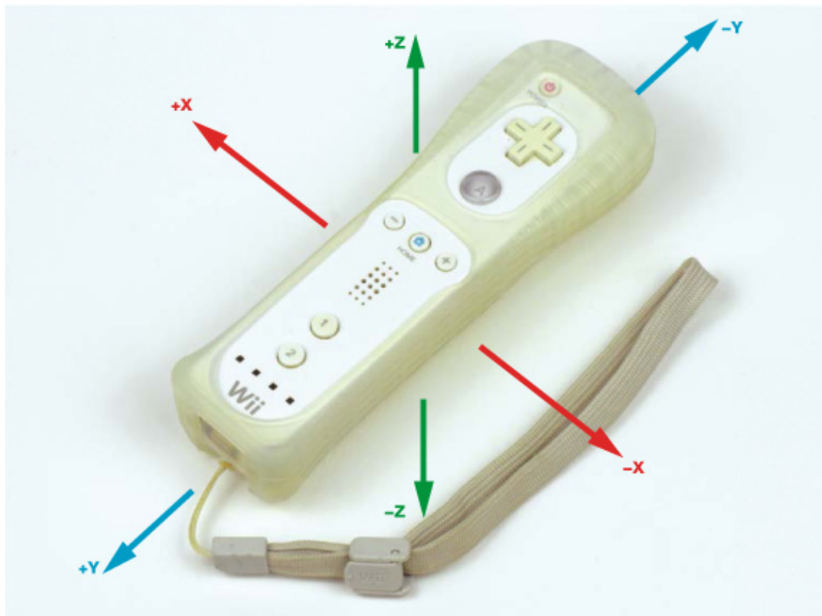
FIGURE 4-8 The axes of motion the Wiimote’s accelerometer can detect
