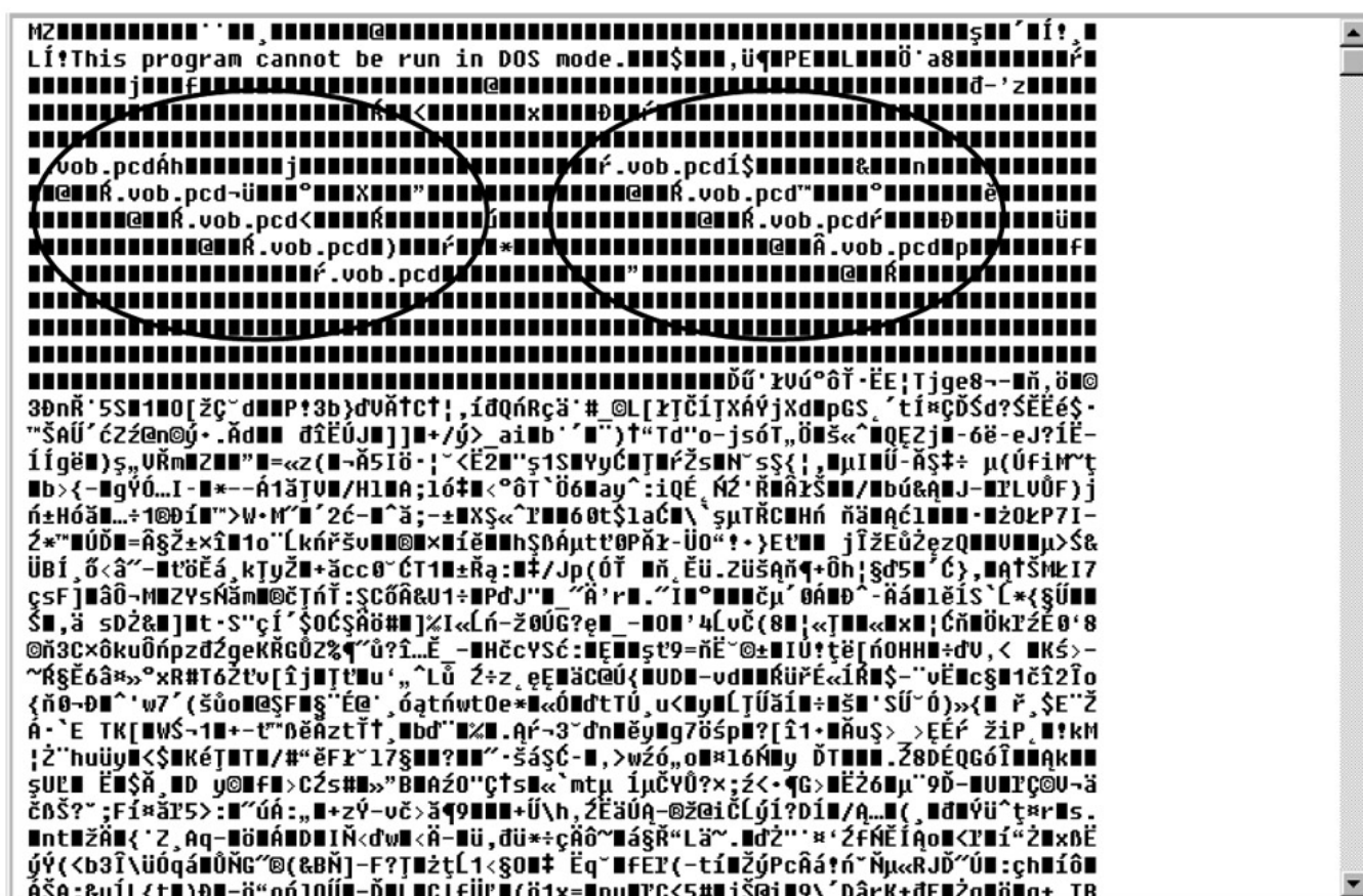
Figure 4.2: VOB is given away by the section name in the PE file header
