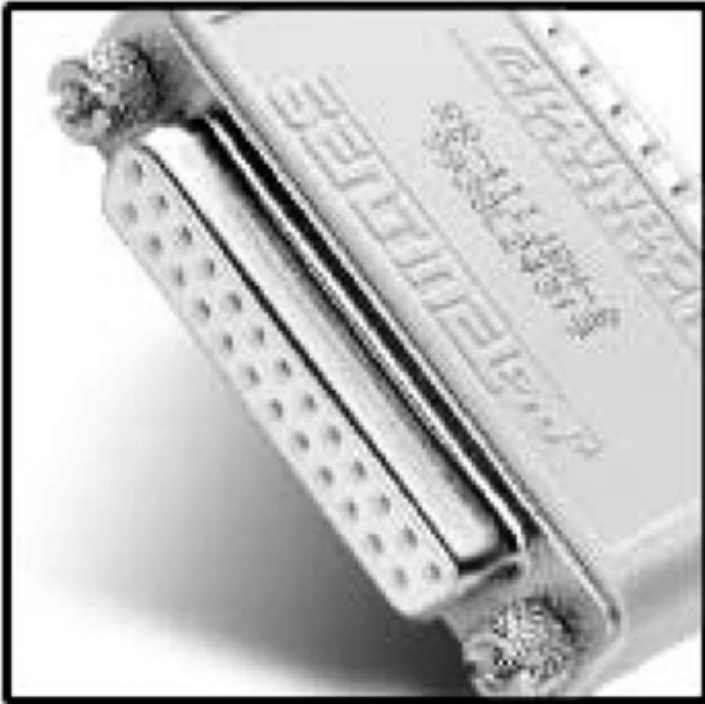
Figure 3.17: There are several kinds of Sentinel hardware keys
