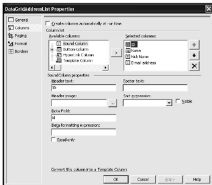
Figure 8-3: The Property Builder of the DataGrid control.
