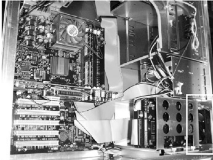
Figure 5-6: Proper fan placement
