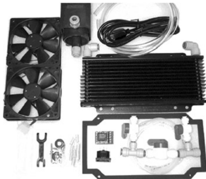
Figure 5-10: SwiftTech liquid cooler
