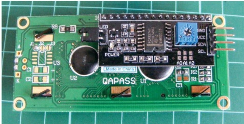
3. Carefully add a small amount of solder to each of the pins to make a connection and hold the serial monitor to the screen. Turn to the primer for a quick soldering guide.
