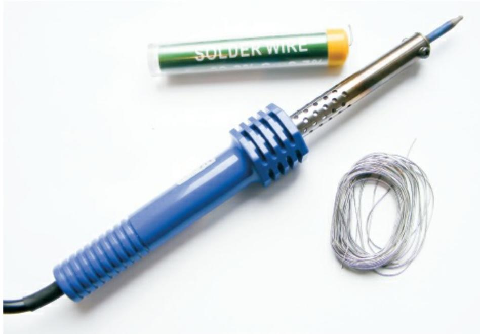
1. Plug in your soldering iron and wait at least 5 minutes for it to reach operating temperature.
