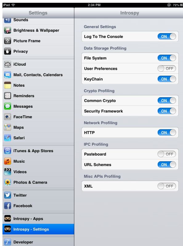
Figure 6-7: The Introspsy settings screen. You can select which applications are profiled on the Apps tab.
