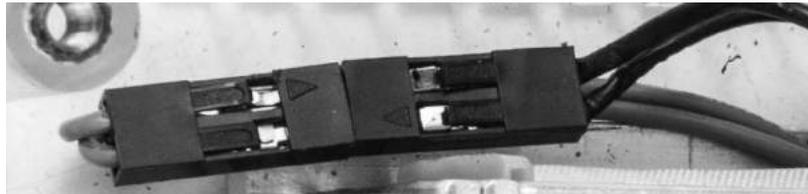
Figure 6-5: A pair of mating connectors used to connect the solenoid
