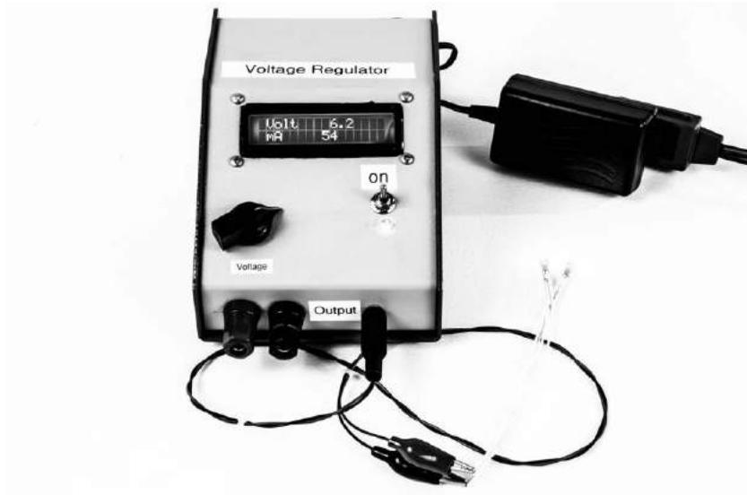
Figure 3-12: The completed Regulated Power Supply
