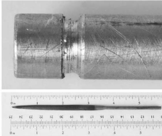
Figure 6-18: A close up of the release groove in the bottom of the release rod (top) and the small needle file used to make the groove (bottom)
