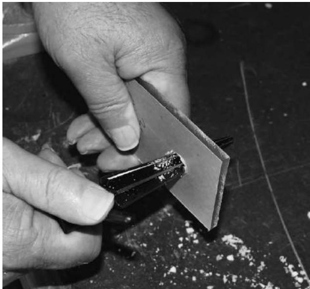
*Figure 4-13: Using a tapered reamer to enlarge the bearing hole to the finished dimension*
