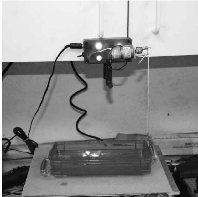
*Figure 2-14: For larger PCBs, try etching in a tray for a more conventional approach. Just attach the motor reverser to your tray to agitate the board rather than using the reverser to dip the board in and out of the solution.*
