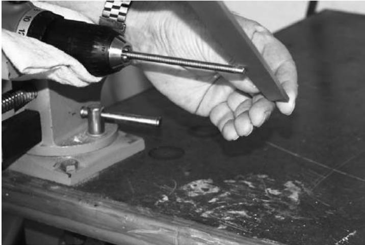
*Figure 4-16: Reducing the diameter of the threaded shaft*
