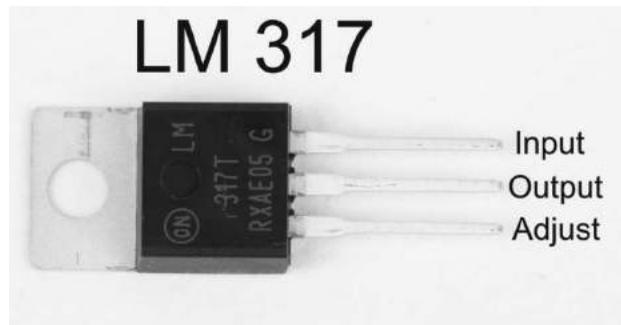
Figure 3-4: Pinout of the LM317 regulator
