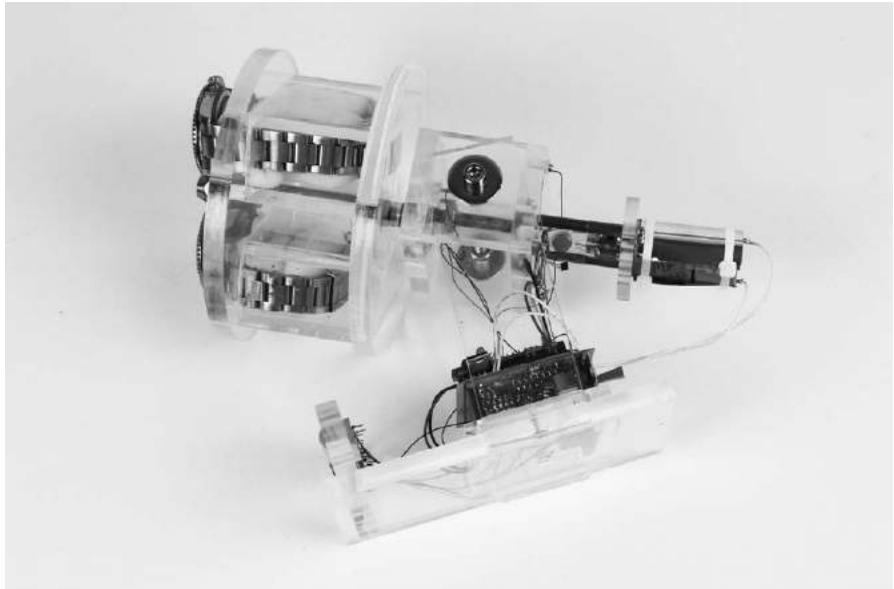
*Figure 4-15: The completed Watch Winder on its side, showing the base fabrication, bearing box, motor mount, and watch basket*
