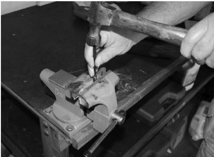
*Figure 4-17: Clamp the shaft of the piece used as the bushing in a vice or pair of vise-grip pliers, and center punch a mark before drilling the hole. Get as close to the center as possible.*
