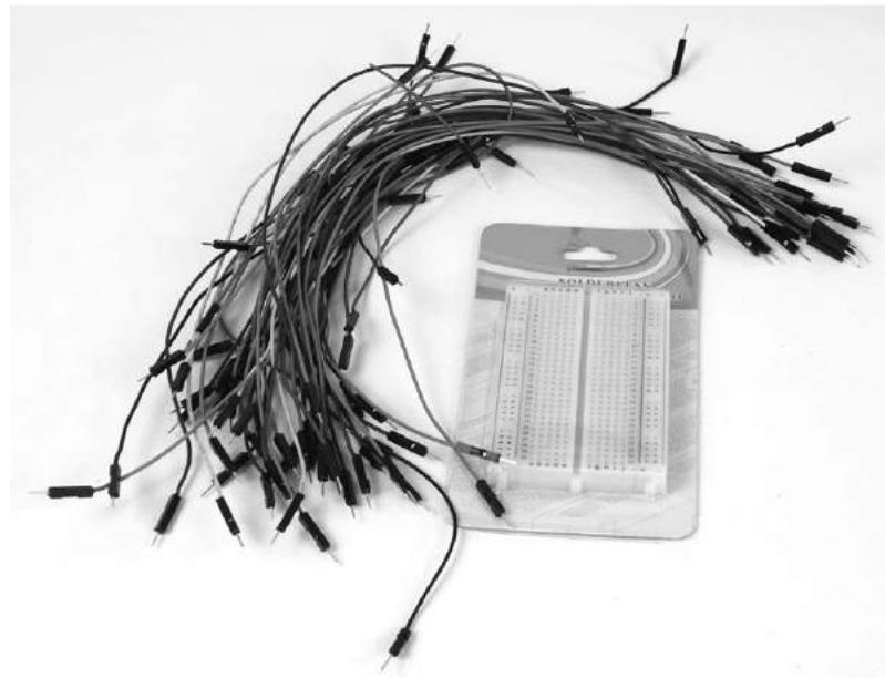
Figure 2-8: Typical small breadboard and plug-in wires
