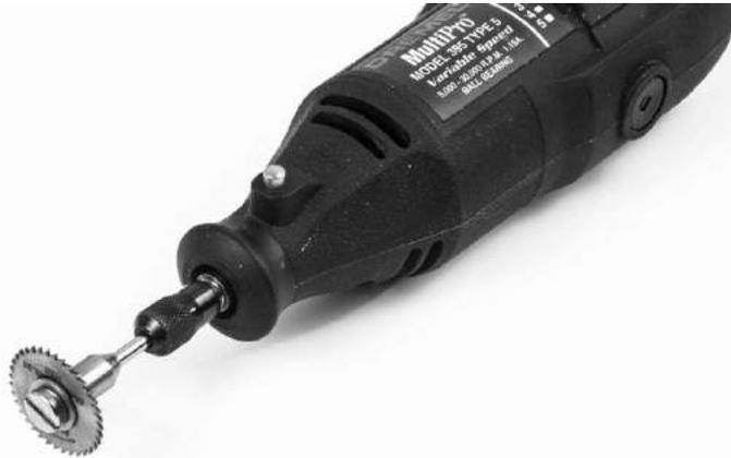
*Figure 6-23: Dremel tool with small circular saw blade attached*
