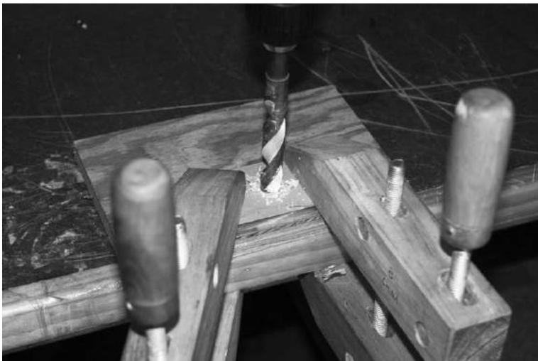
*Figure 4-12: Drilling a large hole in the acrylic. Note that the acrylic piece is securely clamped down.*
