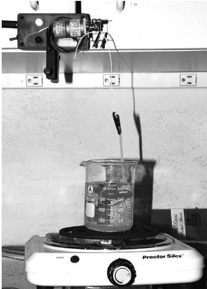
*Figure 2-22: This Arduino-based etcher-agitator etches a board. The etchant should turn emerald as the copper is etched. The board is held by a wire tie that is attached to a wire by an alligator clip. The wire goes through a hole in the crank and is held in place with another alligator clip. One of the LEDs is lit.*
