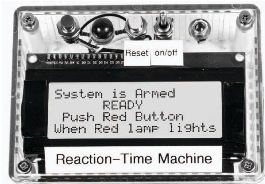
Figure 1-7: The completed Reaction-Time Machine mounted in the Hammond 1591 STCL clear plastic enclosure
