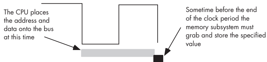
Figure 6-18: A typical memory write cycle
