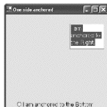
Figure 9-6: Before resizing a form with a text box anchored to the right and a radio button anchored to the bottom
