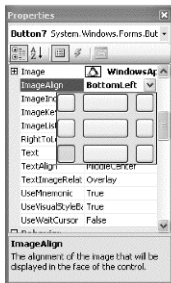
Figure 8-15: Click a position in which your image will appear inside a control.
