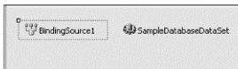
Figure 28-16: As soon as you bind a database to a Visual Basic project, Visual Basic Express automatically creates a dataset control, which links your program to a database file.
