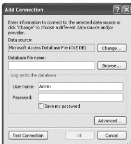
Figure 28-3: The Add Connection dialog box lets you choose a specific database file to include in your Visual Basic program.
