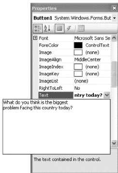
Figure 7-7: If a property holds a large amount of text, such as the Text property, a pop-up window may appear when you double-click the property.
