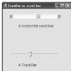
Figure 15-4: A TrackBar displays a fixed number of tick marks to which the slider can point.
