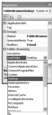
Figure 17-5: The RootFolder property defines which folder initially appears in the Folder Browser dialog box.
