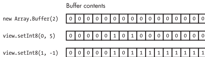
Figure 10-1: The array buffer after two method calls
