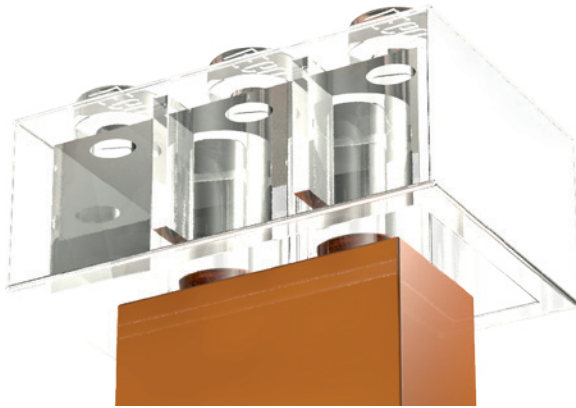
Figure 1-21: Studs inserted into tubes, not alongside them
