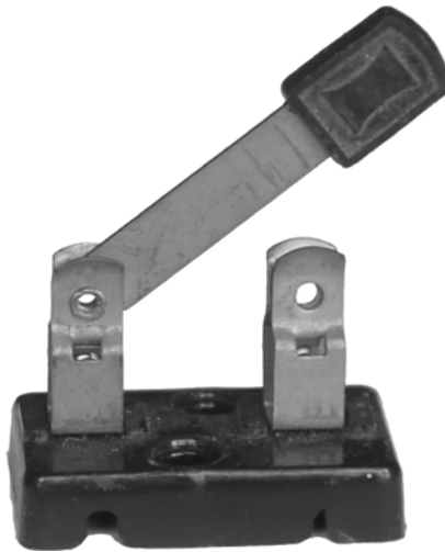
Figure 2-14: Single-pole, single-throw knife switch
