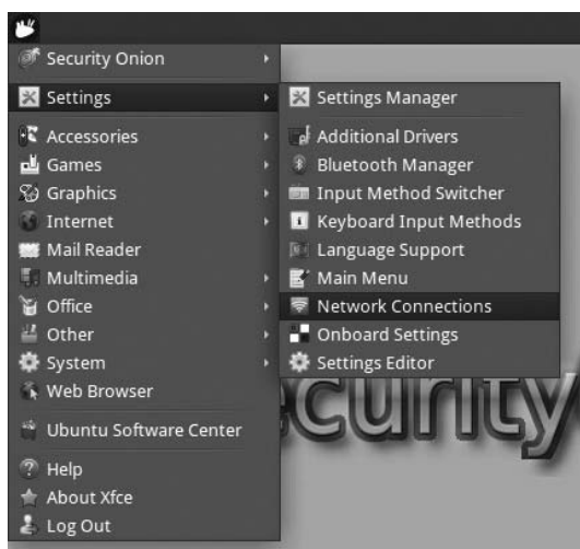
Figure 4-1: Selecting to view settings for Network Connections
