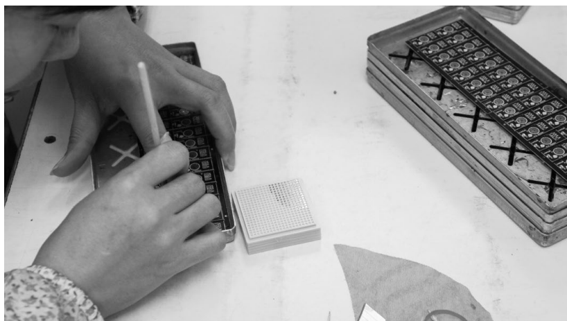
A controller IC being placed on a panel of USB-stick PCBs. The tiny bare dies are on the right, sitting in a waffle pack.
