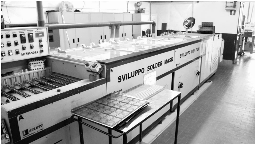
The machine that develops the photoresist
