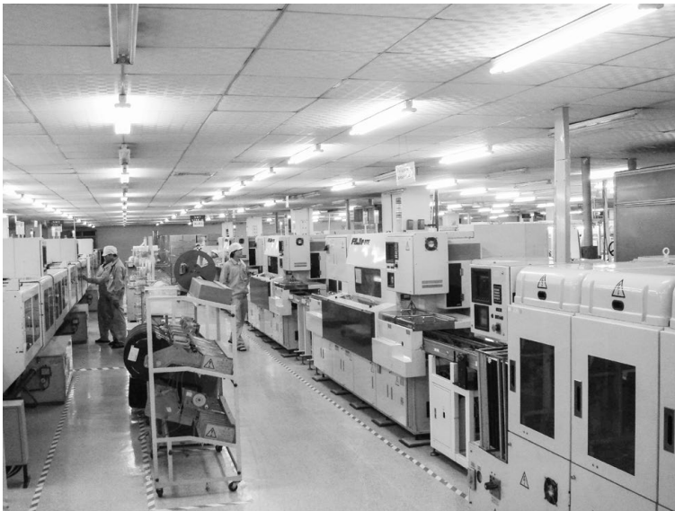
The chumby PCB assembly factory in China had dozens of lines filled with tried-and-true Fuji chip shooters.
