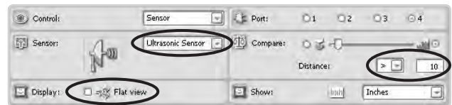
Figure 7-25: Detecting an opening using the Ultrasonic Sensor
