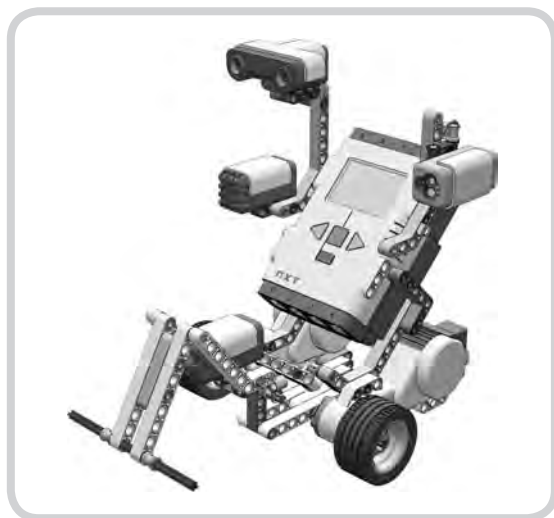
Figure 8-3: The Ultrasonic Sensor pointing to the front of the TriBot
