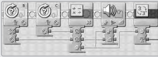
Figure 8-26: The data wires redrawn after closing the Sound block's hub
