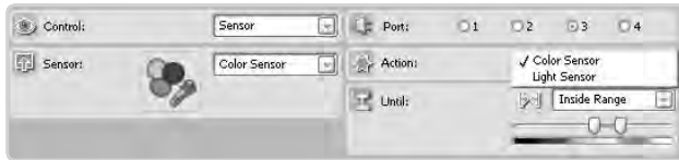
Figure 5-22: Using the Color Sensor as a Light Sensor
