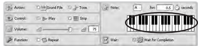
Figure 8-15: Setting the tone using the Configuration Panel
