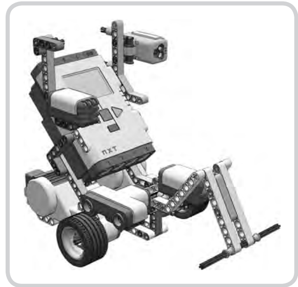
Figure 7-10: The TriBot with the Ultrasonic Sensor pointing to the side
