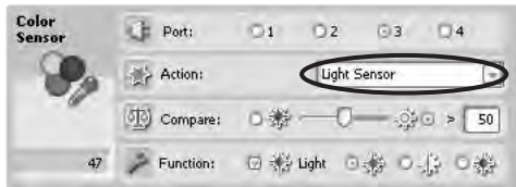
Figure 18-54: Reading the light level using the Color Sensor
