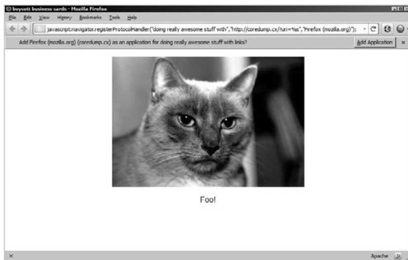
Figure 17-1: A seriously confusing prompt in Firefox. The prompt shown in the upper area of the browser window was generated by the browser in response to a call to the registerProtocolHandler(...) API, with the protocol name set to “doing really awesome stuff” and application name set to “Firefox (mozilla.org)”. This particular example is harmless, but more sinister abuse is within reach.
