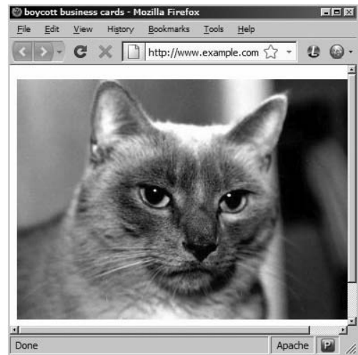
Figure 14-2: A window carefully sized by a script so that the real origin of the displayed content is elided in a confusing way. The actual URL of this cat-themed page is http://www.example.com.coredump.cx/ , not http://www.example.com/ .
