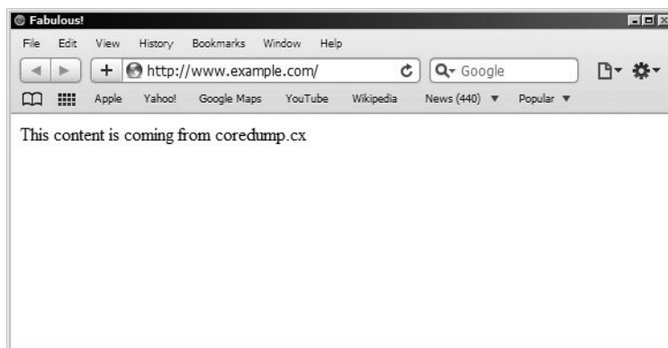
Figure 14-4: Allowing websites to hide the address bar in Safari is a bad idea. The displayed document is not retrieved from http://www.example.com/ . Instead, the page simply displays a screenshot of a real address bar in a window created by window.open("http://coredump.cx/...", "location=no") .
