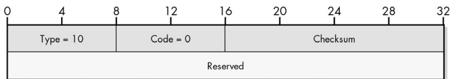
Figure 33-4: ICMPv4 Router Solicitation Message format
