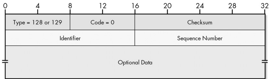
Figure 35-1: ICMPv6 Echo Request and Echo Reply message format
