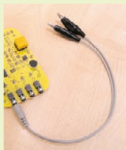
An alligator clip connected to Input A
