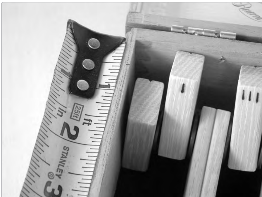
FIGURE 6-7: Measuring the clearance for the scoring tiles
