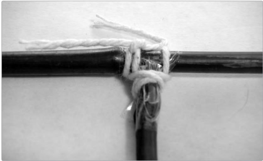
FIGURE 23-18: Wrap the cross braces' joints with string.
