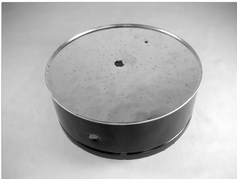
FIGURE 13-9: The cookie tin, drilled to accommodate the bridge bolt (through the hole in the center of the silver bottom), pickup wires (through the small hole located at one o'clock), and the jack (which will be installed in the hole on the side of the tin)
