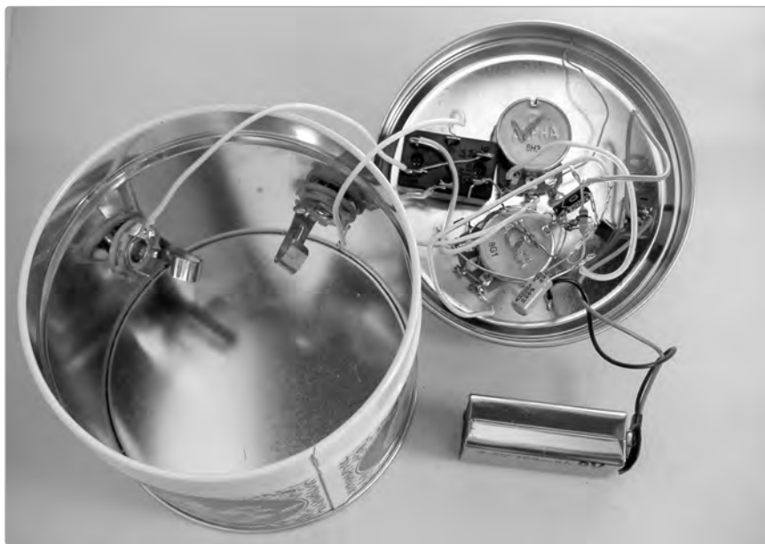
FIGURE 16-10: The packaged Two-Transistor Fuzztone, guts revealed
