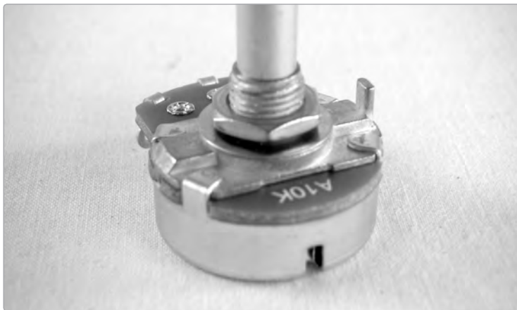
FIGURE 17-12: A close-up of a potentiometer's anchor
