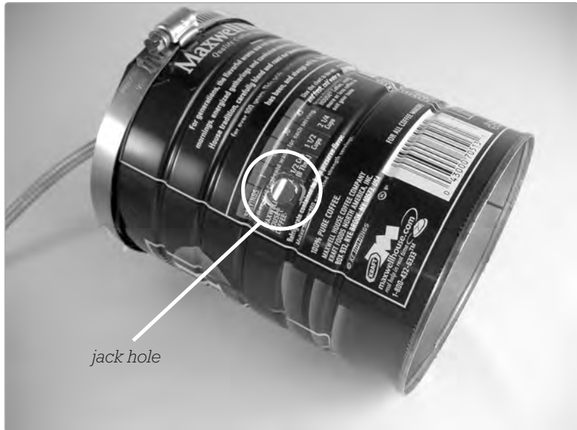
FIGURE 10-9: The drum, with jack hole
