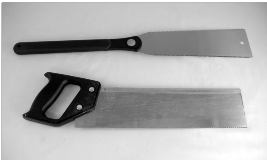
FIGURE 1-8: A conventional crosscut saw (bottom) and a ryoba (top)
