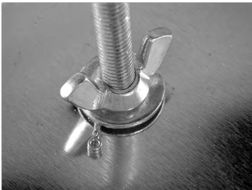
FIGURE 13-10: Locking the string into place
