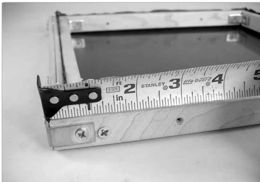
FIGURE 9-9: Measuring for a secondary securing screw
