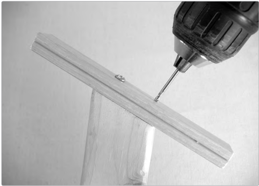
FIGURE 24-6: Drilling a guide hole in the grip
