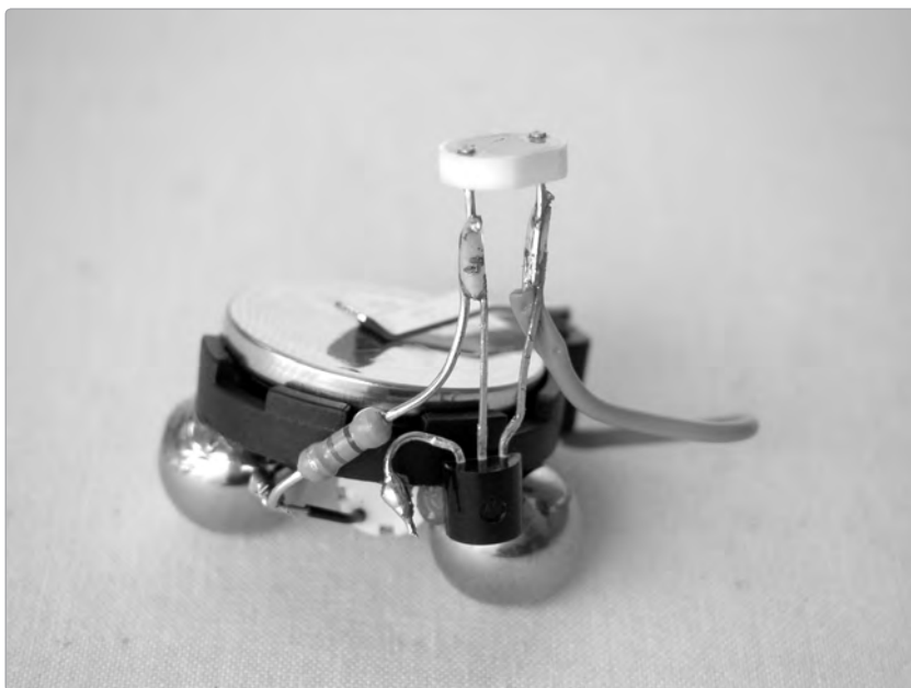
FIGURE 22-11: The back of the finished Jitterbug, showing the configuration of the brain's resistor, transistor, and photoresistor
