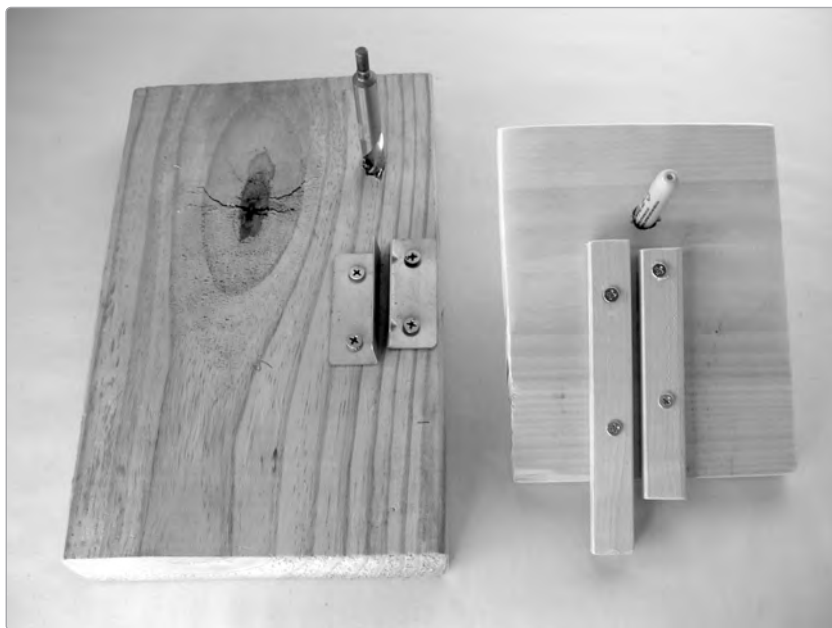
FIGURE 21-4: Here are two versions of the simple pipe-bending jig. The one on the left is made from a pair of shelf brackets and uses a 1/2" drill bit as the bending guide; it makes a counterclockwise coil. The jig on the right is scrap wood, with a Sharpie marker slid through a 1/2" hole in the board as a bending guide, and makes a clockwise coil. Both work great.
