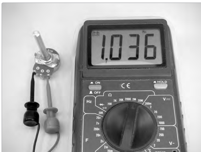
FIGURE A-23: Identifying a potentiometer
