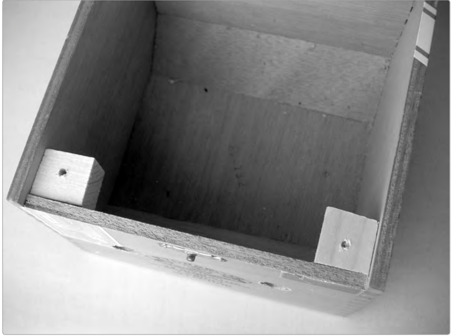
FIGURE 2-4: The blocks installed, with guide holes drilled
