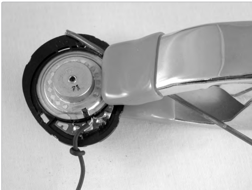
FIGURE 11-13: The pickup, glued and clamped
