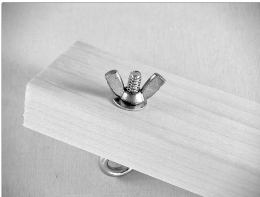
FIGURE 13-8: The homemade tuning peg installed, viewed from the back
