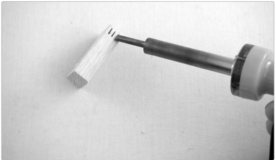
FIGURE 6-5: Numbering a scoring tile with a soldering iron
