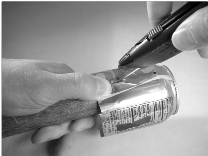
FIGURE 19-6: Using a broom handle for support while adding a cutout
