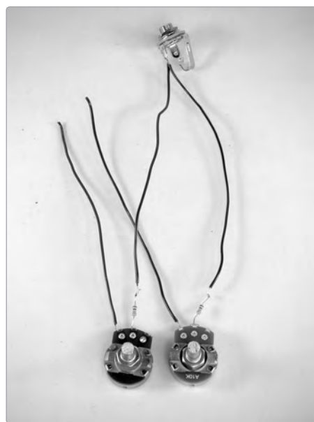
FIGURE 14-4: The reverb's two-channel mixer
