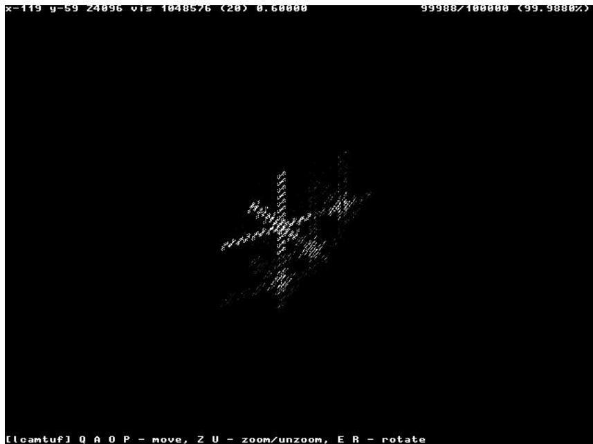
Figure 10-8: HP/UX 11. A strange x-wing structure, 18 bits wide but obviously irregular, likely a sign of high-correlation levels of a flawed PRNG
