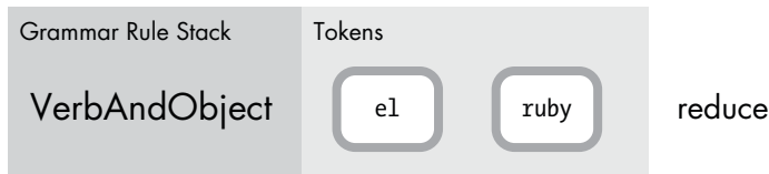
Figure 1-20: The parser reduces again, matching the VerbAndObject rule.
