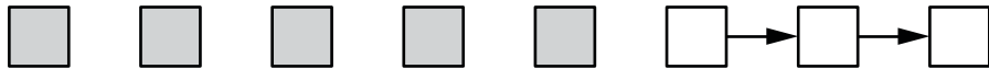
Figure 12-3: As your program creates more objects, MRI starts to use up the free list.
