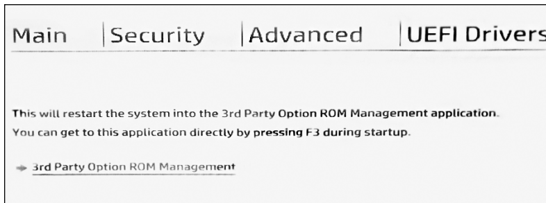
Figure 15-5: Blocking third-party Option ROMs in the BIOS management interface
