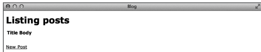
Figure 2-2: The Rails Post scaffolding
