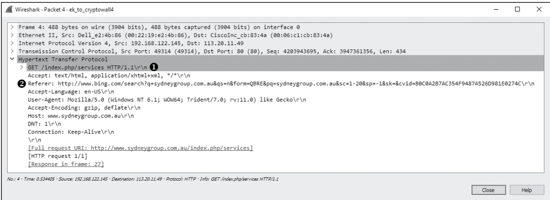
Figure 12-35: An HTTP request to an unknown external host
