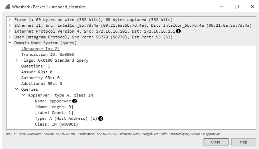
Figure 10-30: Communication begins with a DNS query for the appserver A record.
