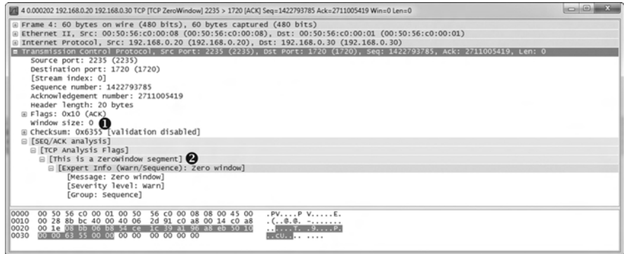
Figure 9-17: This zero window packet says that the host cannot accept any more data.
