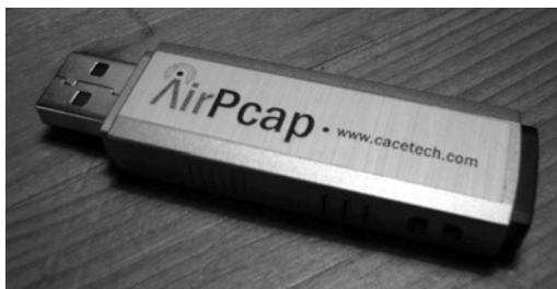
Figure 11-5: The AirPcap device is very compact, making it easy to tote along with a laptop.
