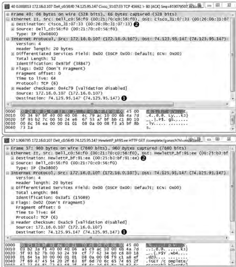
Figure 10-18: The change in target MAC address shows this attack was a success.
