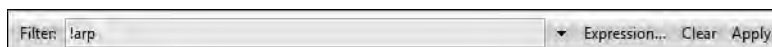
Figure 4-12: Creating a display filter using the Filter text box above the Packet List pane
