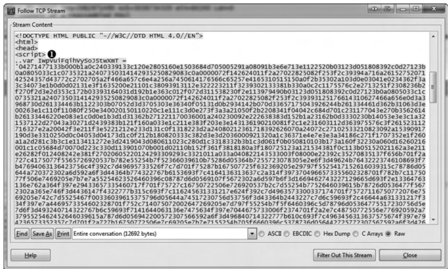
Figure 10-11: This scrambled content within a <script> tag appears to be encoded.
