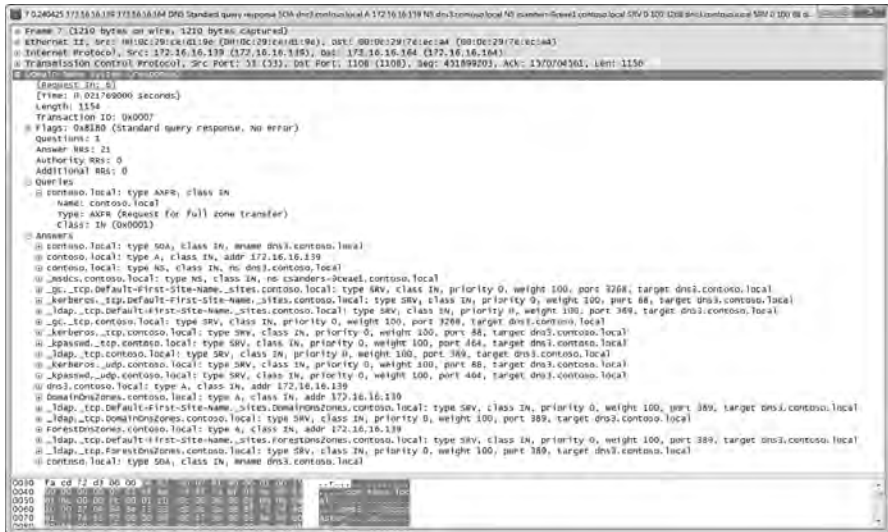
Figure 7-17: The DNS full zone transfer occurring
