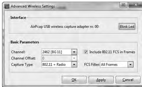
Figure 11-8: The Advanced Wireless Settings dialog allows you to configure AirPcap from within Wireshark.
