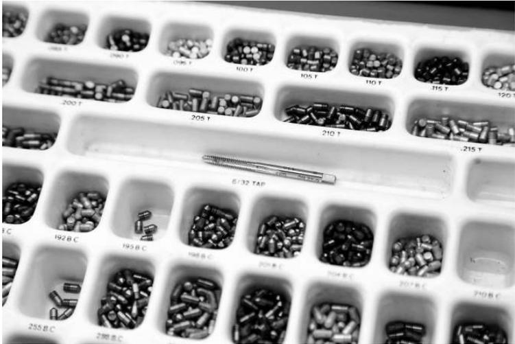
If you have the knowledge of even basic lock field-stripping, it is quite possible to upgrade a pin tumbler lock using this technique for very little cost. The LAB company's S-pins are available for less than a dime each<sup>15</sup> and hardware tool suppliers sell both the 6/32" tap and a suitable tap handle for four dollars apiece.
