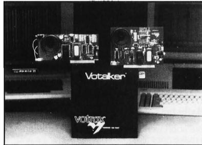
Votalker IB and AP are the only Synthetic Speech Generating Systems for Personal Computers that Provide Four Voice Patterns Through On-Board Switches. Both board-level products offer two preprogrammed voice modes that may be further customized through an on-board filter. Voice modes and filter are activated by switches.
