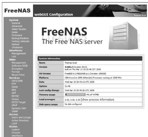
Figure 9-4: FreeNAS is a simple version of Unix designed for use as a file server.
