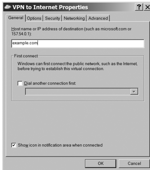
Figure 13-13: The General tab controls the destination of a VPN connection.
