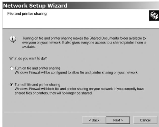
Figure 11-5: Select the file and printer sharing option that applies to your network.
