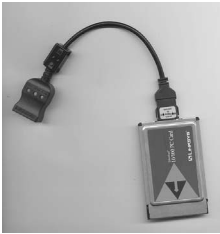
Figure 7-4: This 16-bit PC card network adapter uses a short cable (sometimes called a dongle) to connect the adapter to an Ethernet socket.
