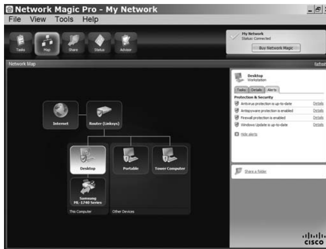
Figure 17-2: Network Magic scans your LAN and displays all the devices connected to it.
