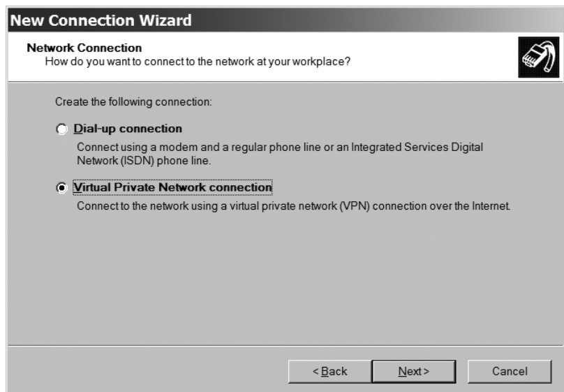
Figure 13-7: Select the Virtual Private Network connection option to create a VPN connection.
