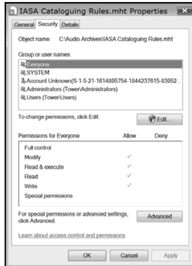
Figure 12-10: The Security tab controls file-sharing permissions for individual files.
