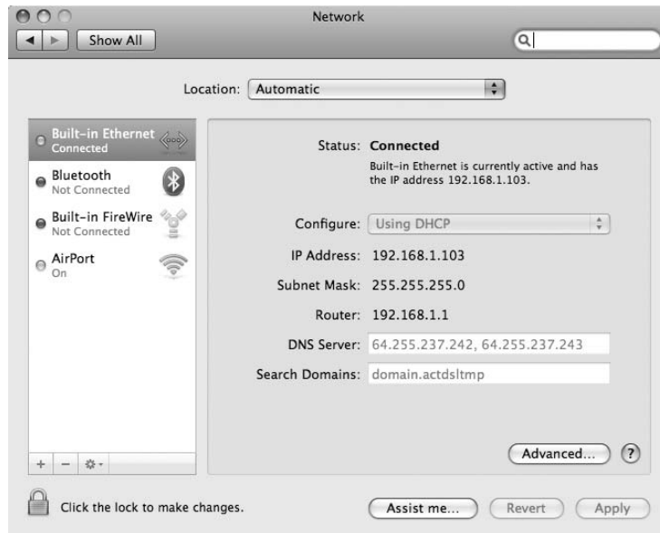
Figure 11-11: The Network window shows the current network connection settings.
