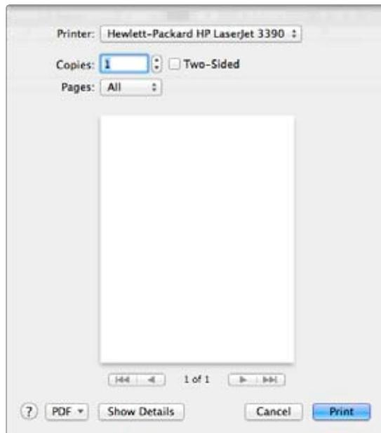
**FIGURE 3-4:** Common parts of a dialog; note that the default button here is the Print button, which is highlighted.
