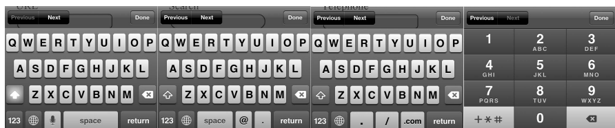
Figure 8-2: The sympathetic soft keyboard on iPhone, optimized for (from left to right) text, email, url, and tel input types
