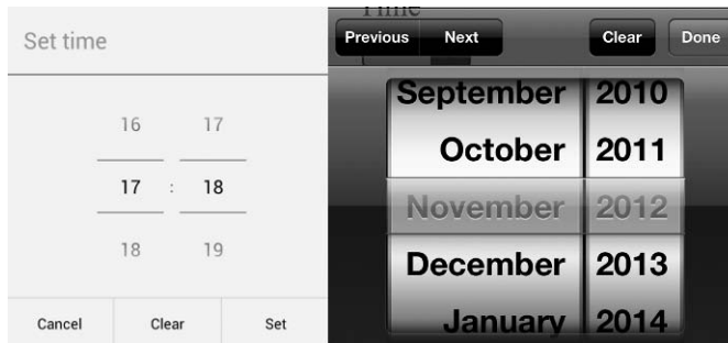
Figure 8-6: A time picker on Chrome for Android (left) and a month picker for iPhone (right)
