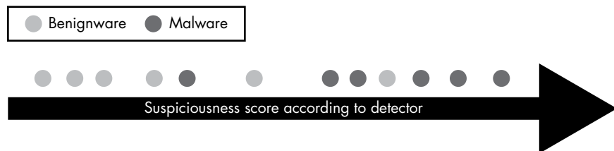
Figure 7-2: Suspiciousness scores output by the hypothetical MalDetect system for individual software binaries
