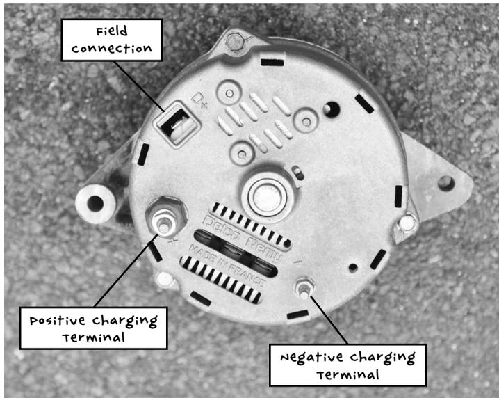
FIGURE 2-16: DELCO LRA443 ALTERNATOR (FROM THE 1980S)
