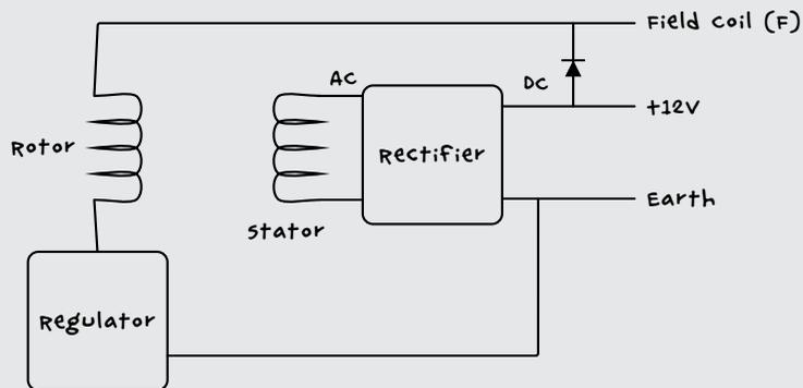
FIGURE 2-13: THE SCHEMATIC DIAGRAM FOR AN AUTOMOTIVE ALTERNATOR
