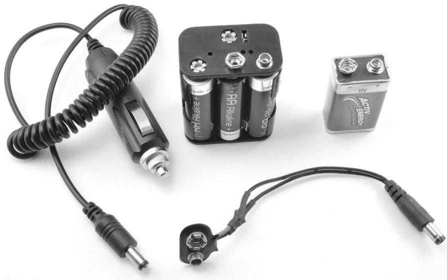
FIGURE 9-10: OPTIONS FOR POWERING THE ARDUINO
