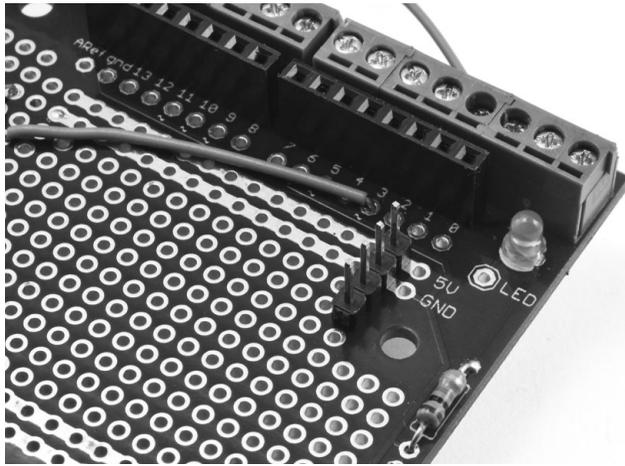
FIGURE 8-8: THE HEADER PINS SOLDERED IN PLACE
