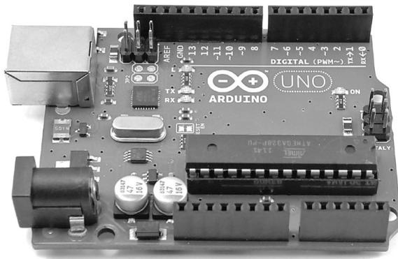
FIGURE 1-5: AN ARDUINO MICROCONTROLLER BOARD
