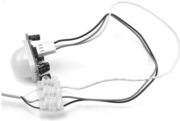
**FIGURE 4-11: PIR LEAD AND TERMINAL BLOCK**
