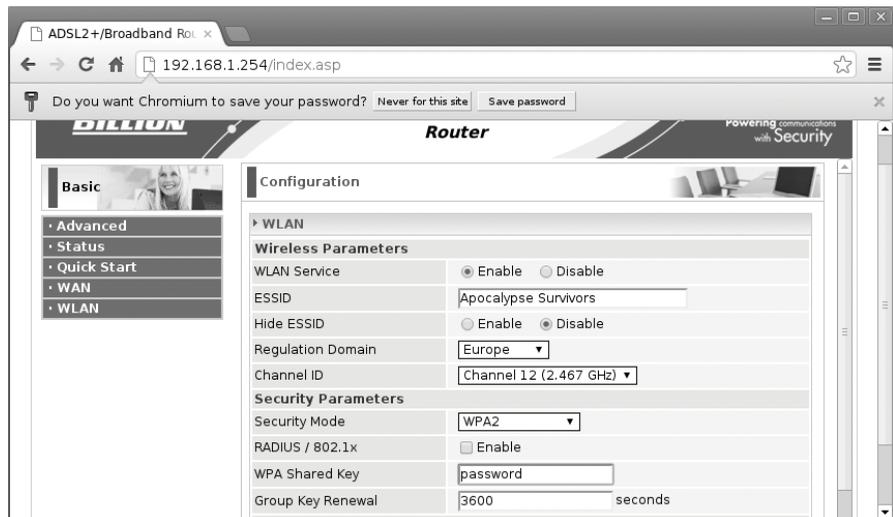
FIGURE 5-12: SETTING UP A WIRELESS NETWORK
