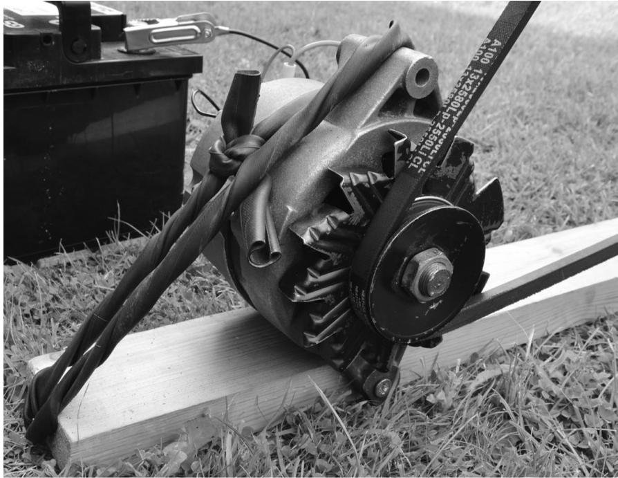
FIGURE 2-15: ATTACHING THE ALTERNATOR TO THE 2X4
