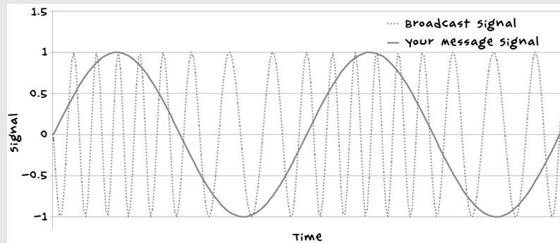
FIGURE 10-3: FREQUENCY MODULATION
