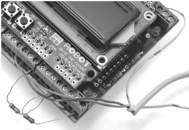
**FIGURE 4-12: CONNECTING THE PIR LEAD TO THE ARDUINO SCREWSHIELD**
