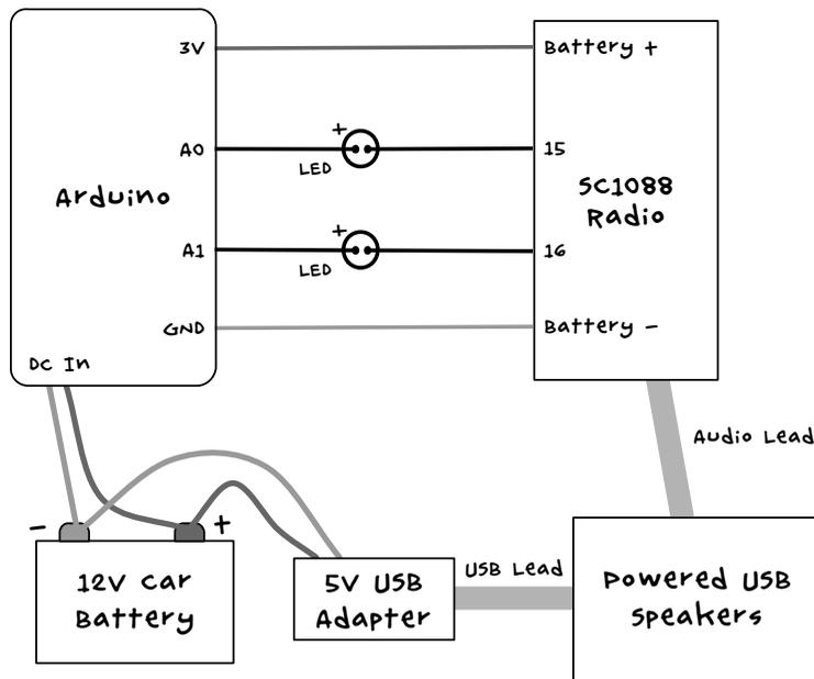
FIGURE 10-6: RADIO SCANNER WIRING DIAGRAM. THE NUMBERS 15 AND 16 ON THE SC1088 RADIO INDICATE PIN NUMBERS OF THE CHIP.
