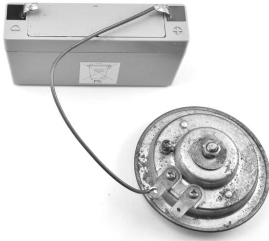
**FIGURE 4-6: CONNECTING THE HORN AND BATTERY**
