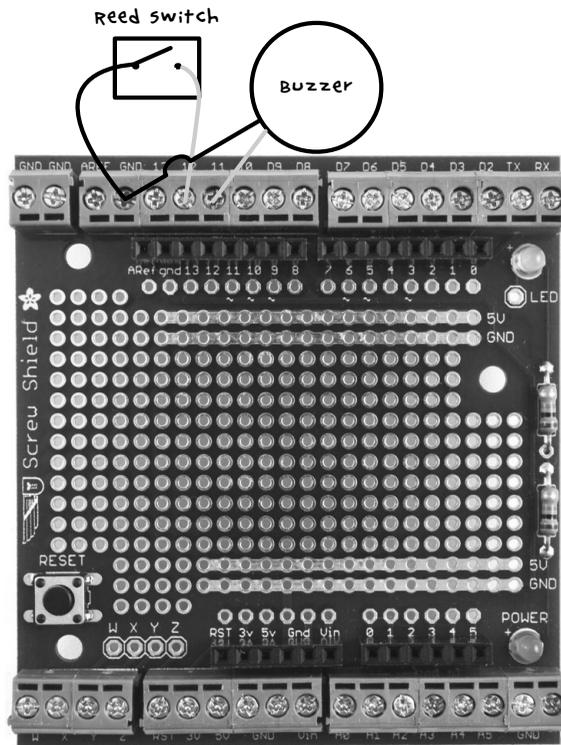
FIGURE 6-13: WIRING DIAGRAM FOR THE DOOR SENSOR
