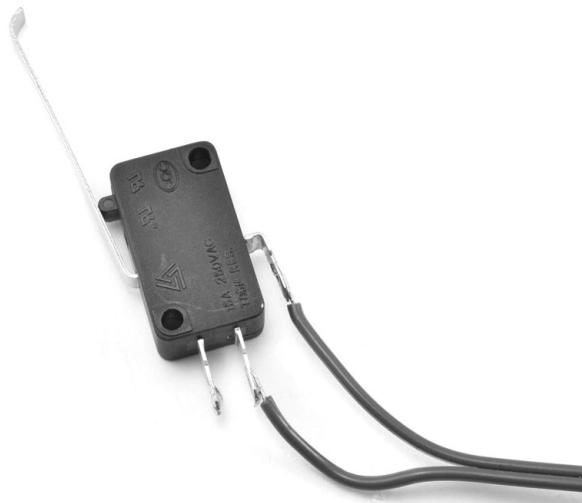
**FIGURE 4-7: SOLDERING WIRES TO THE SWITCH**
