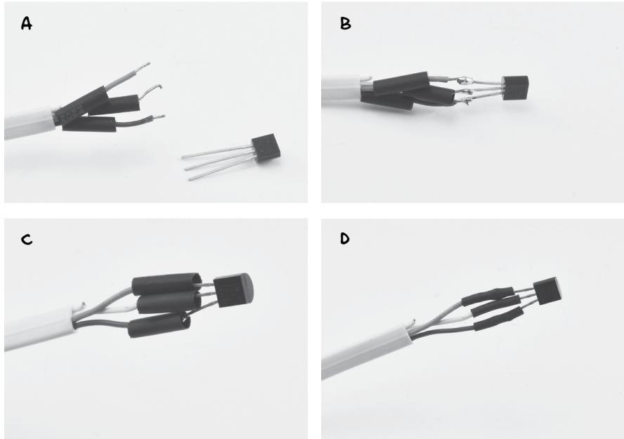
FIGURE 7-14: USING HEATSHRINK ON THE TMP36 LEAD
