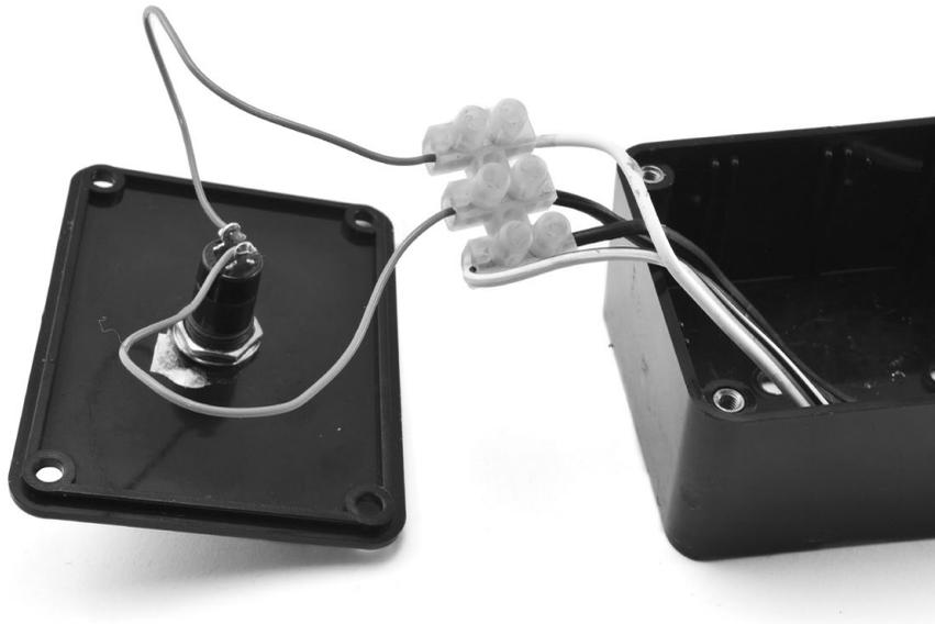
FIGURE 6-9: WIRING UP THE SWITCH BOX
