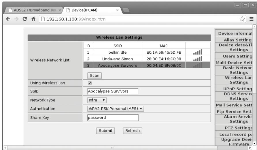
FIGURE 5-14: CONNECTING THE CAMERA TO THE WIRELESS NETWORK
