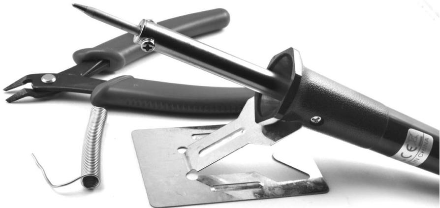
FIGURE B-3: A BASIC SOLDERING KIT
