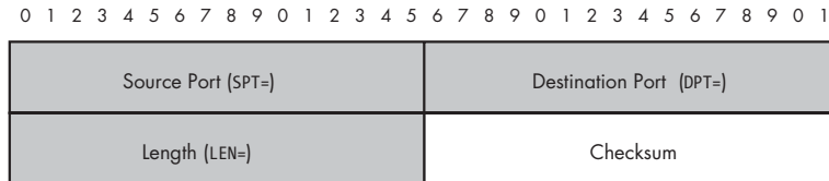
Figure 3-3: The UDP header and iptables log message fields
