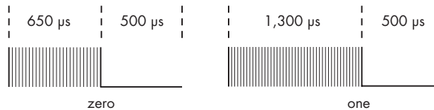
Figure 12-3: Modulated pulses in the Sony TV protocol
