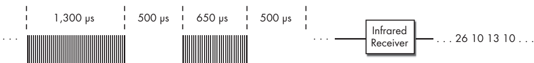
Figure 12-8: Measuring waveform timing in external hardware
