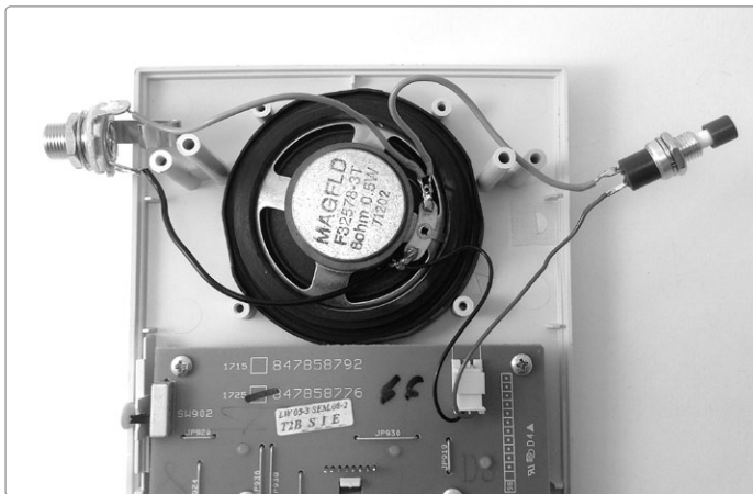
FIGURE 7-7: An auxiliary output with a momentary mute
