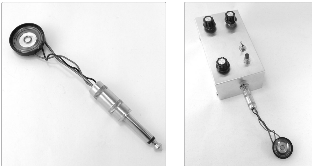
FIGURE 15-17: A simple dandelion speaker for your Single-Chip Space Invader Synth
