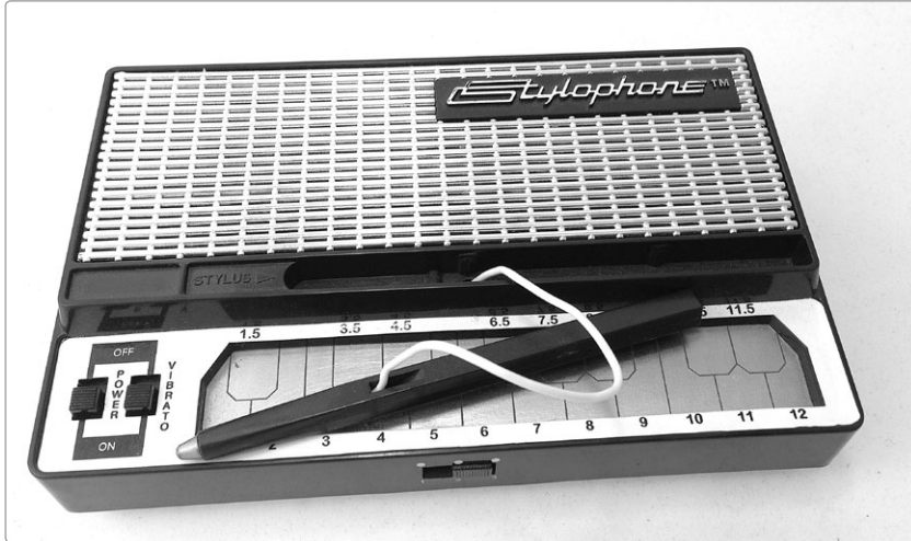
FIGURE 15-21: A commercial Stylophone uses a resistor ladder and stylus for the keyboard control.
