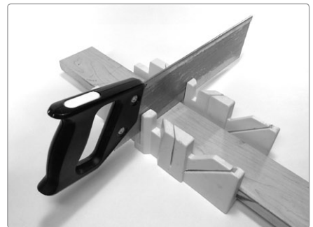
FIGURE 10-7: A miter box is used to cut accurate, precise, reproducible angles (action shot on the right).
