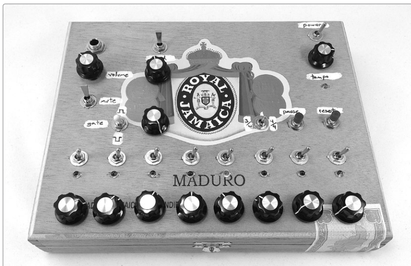
FIGURE 16-1: The finished Bleepbox 8-Step Analog Sequencer
