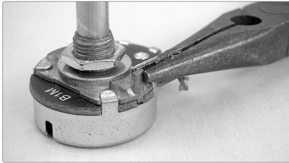
FIGURE A-4: Snapping off the anchor. Quick quiz: what's the maximum resistance this pot offers, and does it have a linear or audio taper? 1
