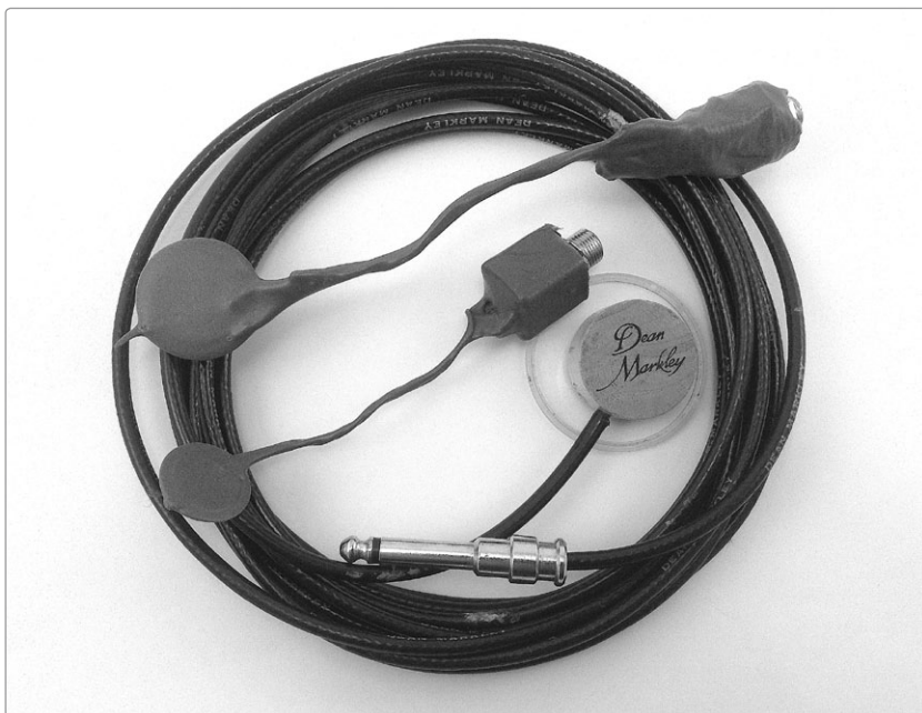
FIGURE 2-9: My pricey Dean Markley acoustical transducer and a couple of homebrew Plasti-Pickups
