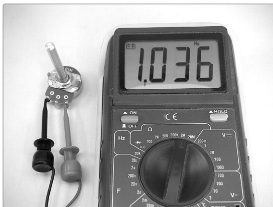
FIGURE A-26: Identifying a potentiometer's resistance
