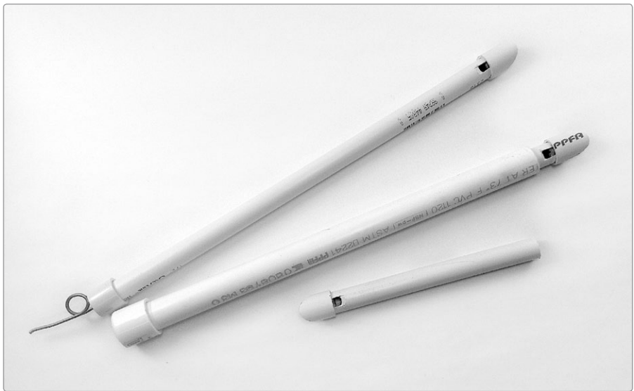
FIGURE 4-19: A finished CPVC Slide Whistle (top), water whistle (middle), and two-tone whistle (bottom)
