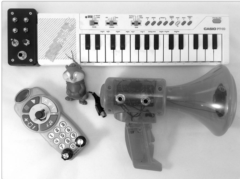
FIGURE 7-1: A selection of circuit-bent instruments and toys. Note the black box on the keyboard and the new bits on the other three: the knobs, switches, and bare metal contacts allow us to tinker with the toys' pitch and tone on the fly, while the jacks allow us to amplify the output (and, in the case of the megaphone, pump our own signal into the input).
