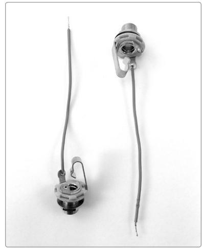
FIGURE 14-6: Input and output jacks
