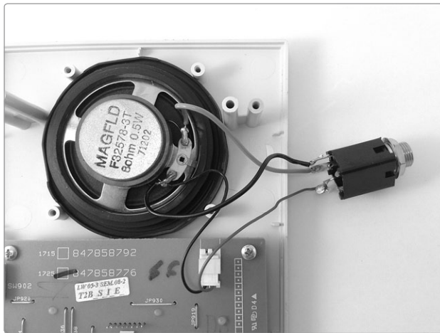
FIGURE 7-8: A finished switch jack output
