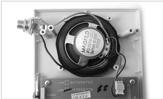
FIGURE 7-6: A “jumpered” auxiliary output jack
