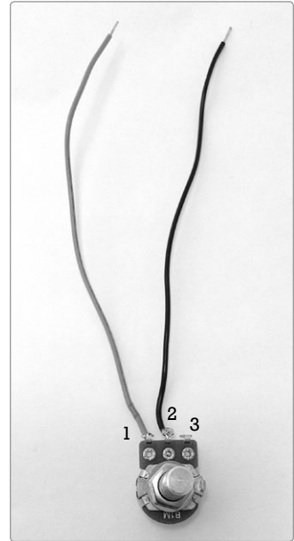
FIGURE 16-6: The prepared tempo control pot
