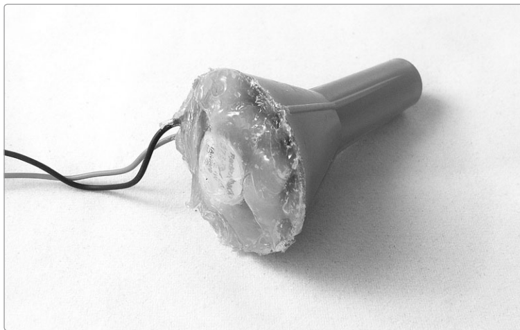
FIGURE 6-17: The glued speaker with a pretty thick layer of insulating silicone
