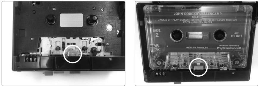
FIGURE 5-3: The elusive play head is circled. On the right, notice the same tape deck from a different angle (including a period-appropriate cassette, for reference).
