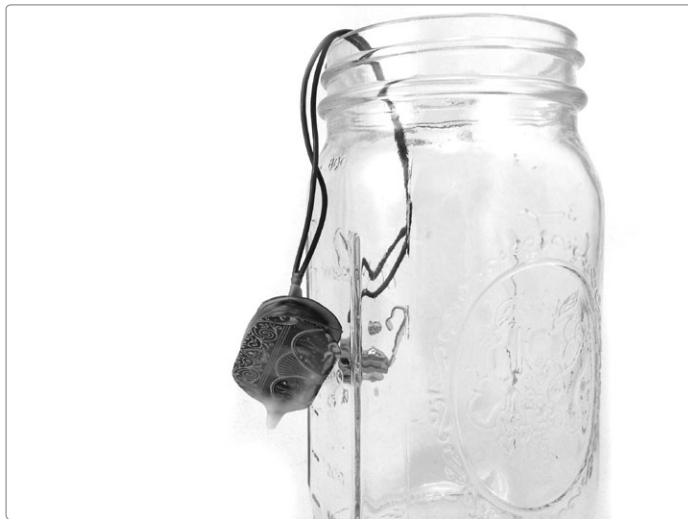
FIGURE 9-8: Drip-drying the potted pickup
