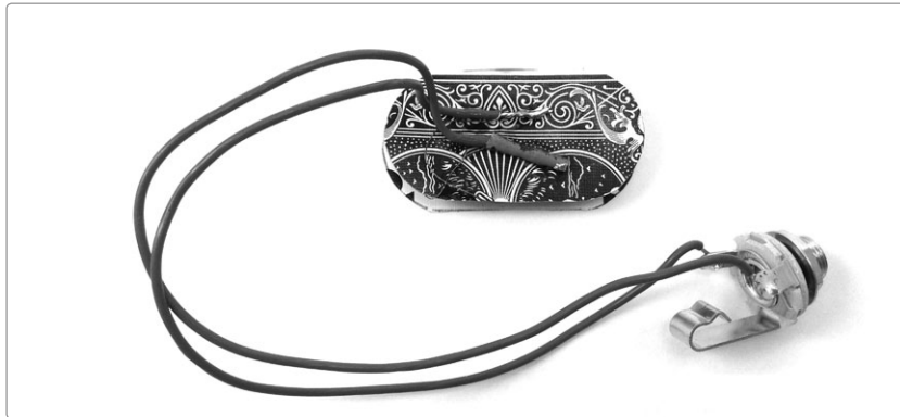
FIGURE 9-7: Fully functional pickup, ready for potting
