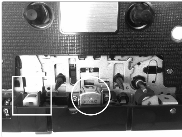
FIGURE 5-4: Play head (circled) and erase head (boxed)
