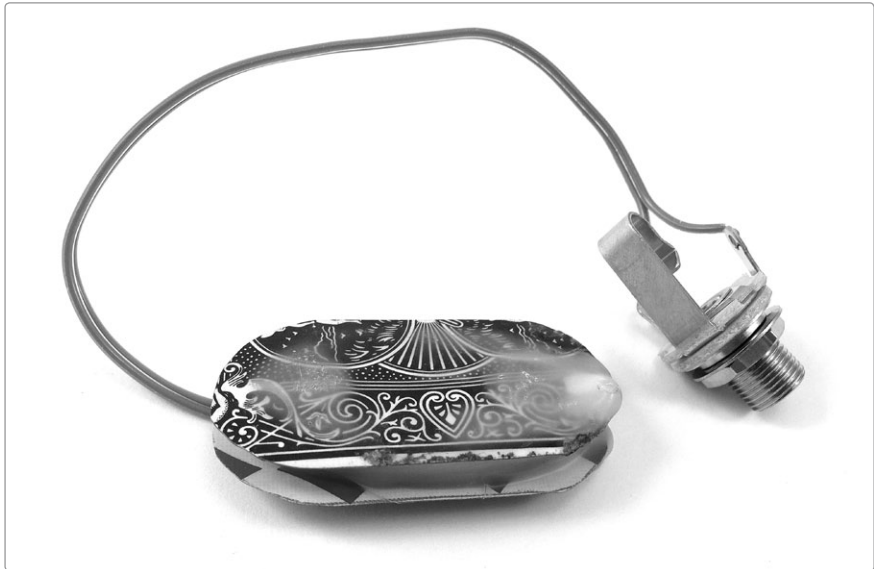
FIGURE 9-1: The finished Playing-Card Pickup
