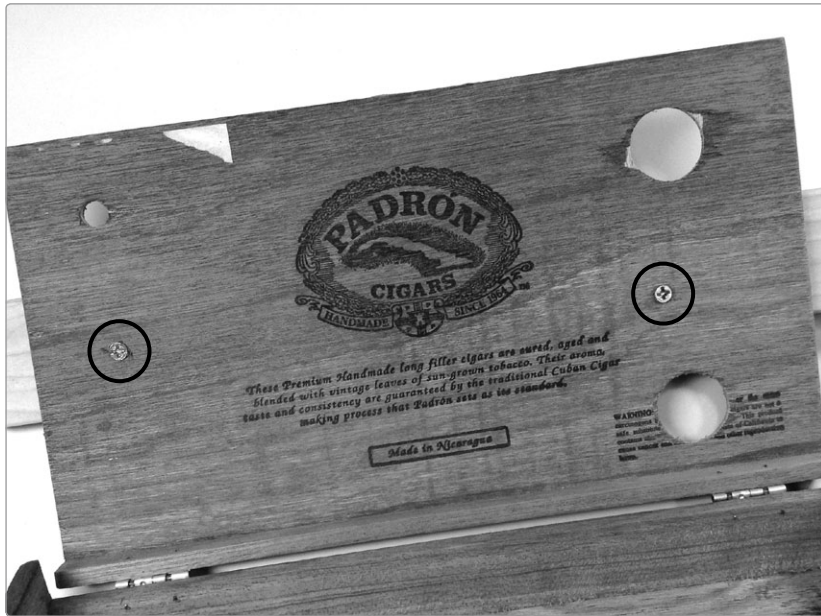
FIGURE 10-14: Anchoring the neck to the uke soundboard (the circles indicate the location of the two neck-mounting screws)
