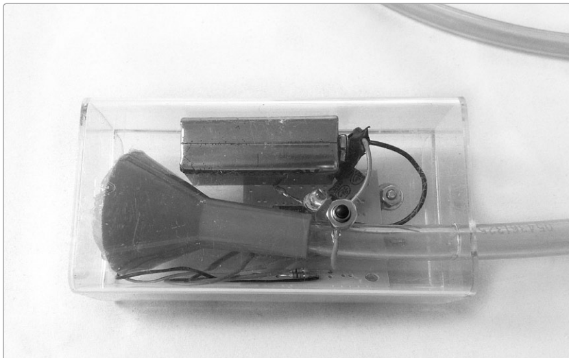
FIGURE 6-20: The finished Droid Voicebox from a different angle, showing off our hacked-together compression driver
