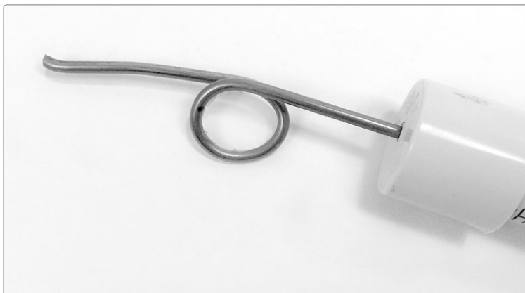
FIGURE 4-17: The finished slide handle
