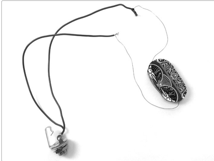
FIGURE 9-6: Leads and jack connected
