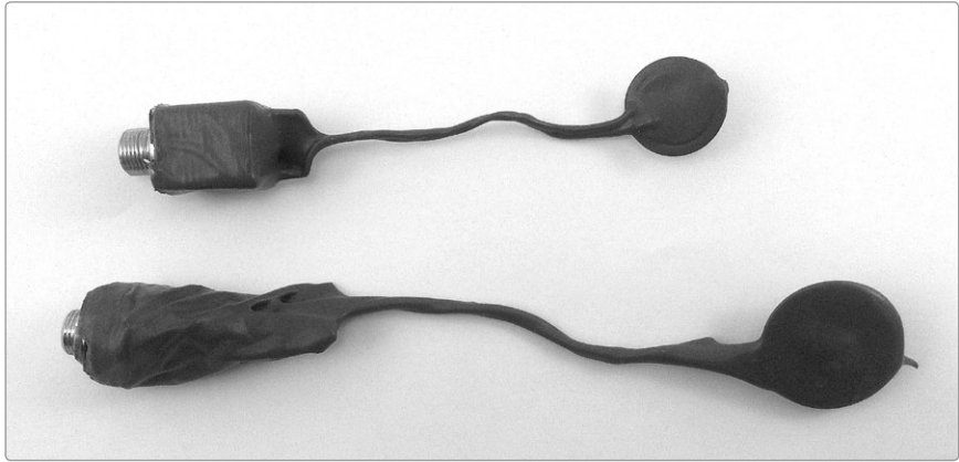
FIGURE 2-10: The top pickup was made using the piezo and partially enclosed jack from the parts list. The bottom was made using a larger piezo element and a regular guitar jack, like the common Switchcraft jack listed for most projects in this book. Both work great!
