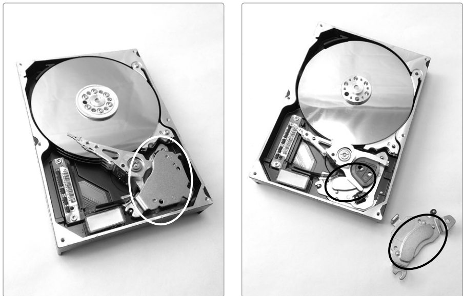
FIGURE 9-9: A broken hard drive with the cover removed (left) and the same drive partially dismantled to reveal the pair of curved neodymium magnets (right). The circles indicate the location of these wonderfully powerful magnets.
