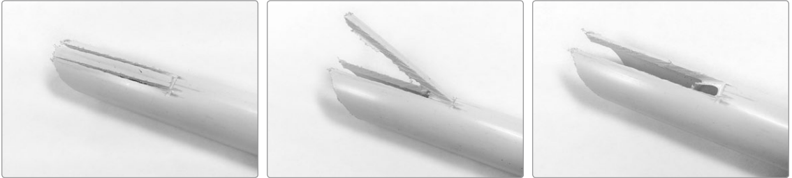
FIGURE 4-9: Your windway is cut (and sloppy)!
