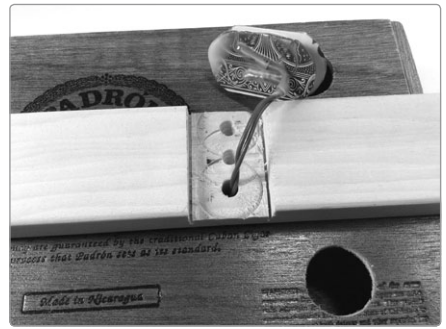
FIGURE 10-15: The hole for my pickup's leads aligns with one of the spade bit's guide holes from Step 11. You can see that more clearly with the pickup wires installed (right).
