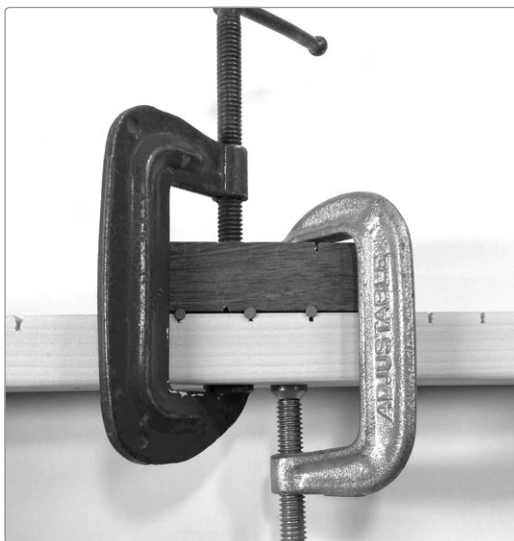
FIGURE 10-9: Pressing the frets into place with a set of clamps
