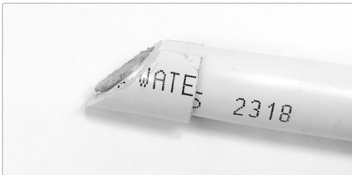
FIGURE 4-16: The slightly protruding fipple block
