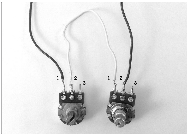
FIGURE 13-21: Daisy-chaining pots to fake your way to higher resistance
