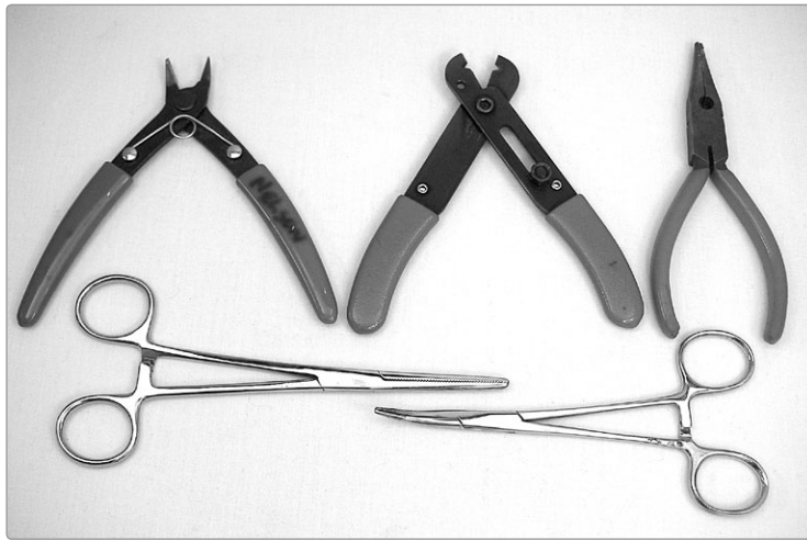
FIGURE A-15: Clockwise from top left: diagonal cutters, wire strippers, needle-nose pliers, and two types of clamps
