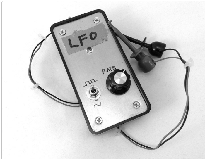
FIGURE 13-1: The finished Universal LFO
