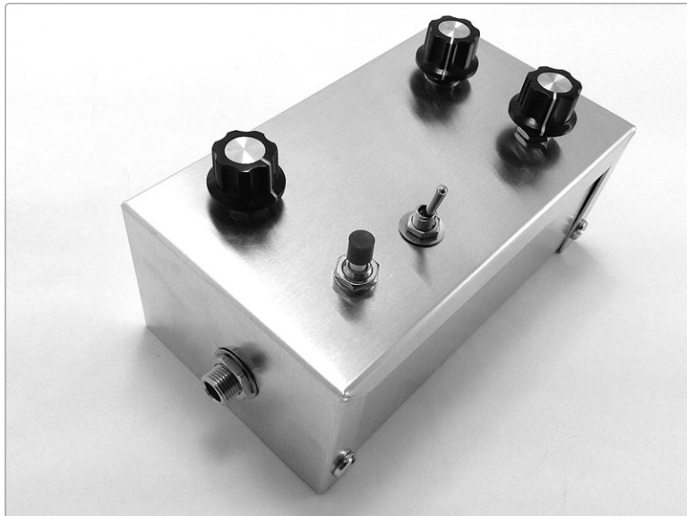
FIGURE 15-1: The finished Single-Chip Space Invader Synth
