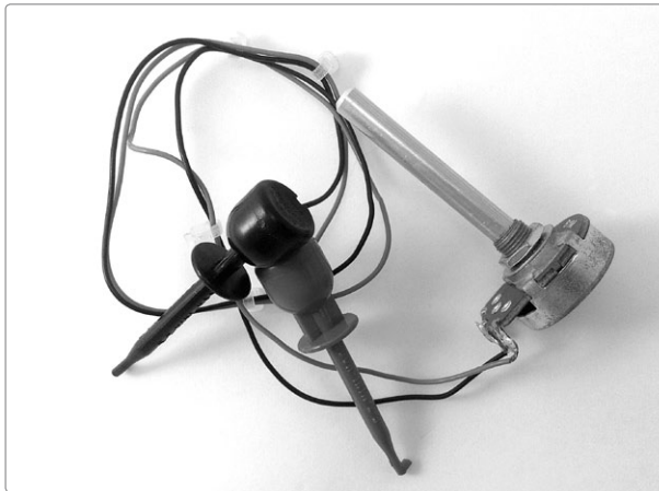
FIGURE 7-12: A clip-on variable resistor
