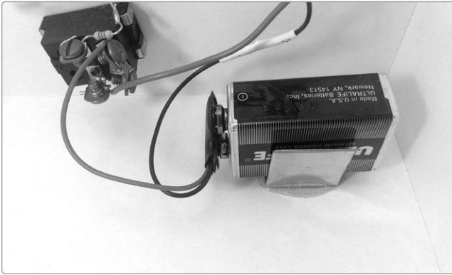
FIGURE 12-20: A 9-volt battery holder clip in a finished project, with and without a battery in place
