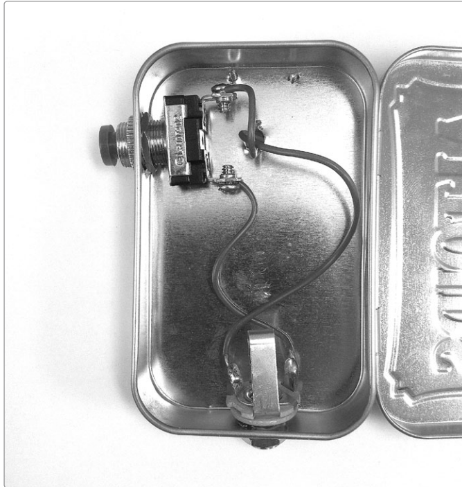
FIGURE 5-13: The guts of your completed Scratchbox. (The play head, which is mounted to the back of the tin, isn't visible. Flip back to Figure 5-12 to see how that fits onto the case.)
