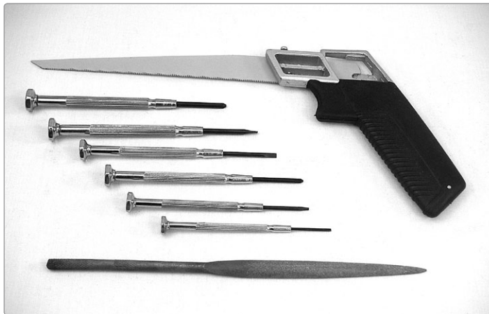
FIGURE A-18: A hacksaw (top), jeweler's screwdrivers (middle), and a tapered half-round file (bottom)
