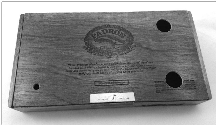
FIGURE 10-13: The sound and jack holes in the cigar-box body
