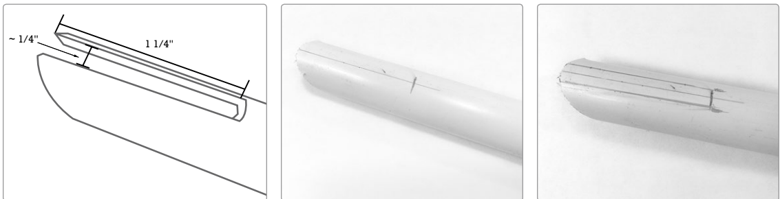
FIGURE 4-6: A diagram of a finished windway slot, including dimensions (left) and guidelines for your windway cuts (middle and right)
