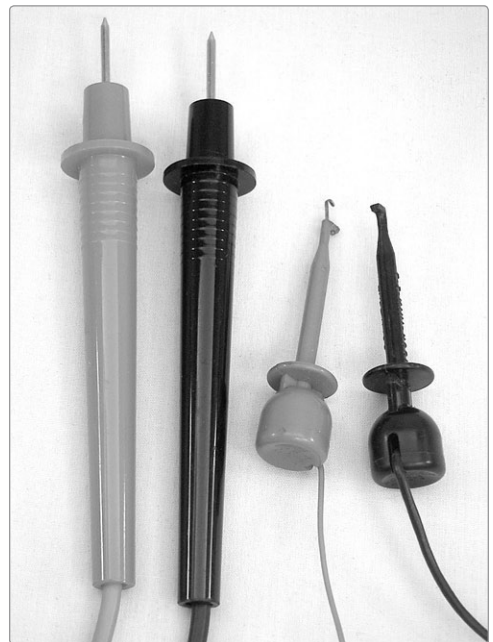
FIGURE A-20: A set of probes (left) and mini-clip leads (right). The latter are retractable hook leads, also called mini-clip jumpers, and are easy to clip to the leg of a single PCB-mounted component without creating a short circuit.
