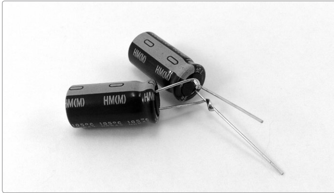
FIGURE 13-22: Stacking caps to fake your way to a higher value
