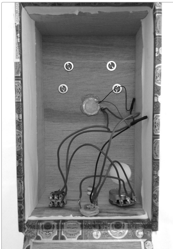
FIGURE 11-20: The guts of the finished Twang & Roar Kalimba. Note the silicone insulating the piezo element.
