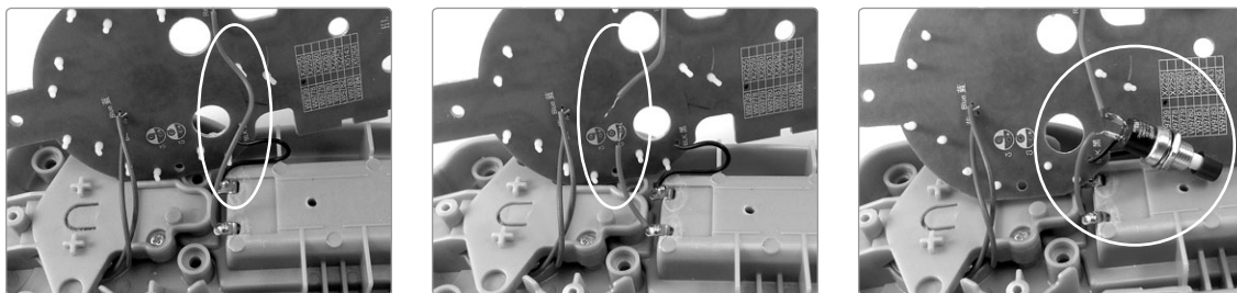
FIGURE 7-18: Installing a momentary power reset switch. Find the power connection (the long wire in the middle of the left image), cut it (center), and solder in the switch (right).
