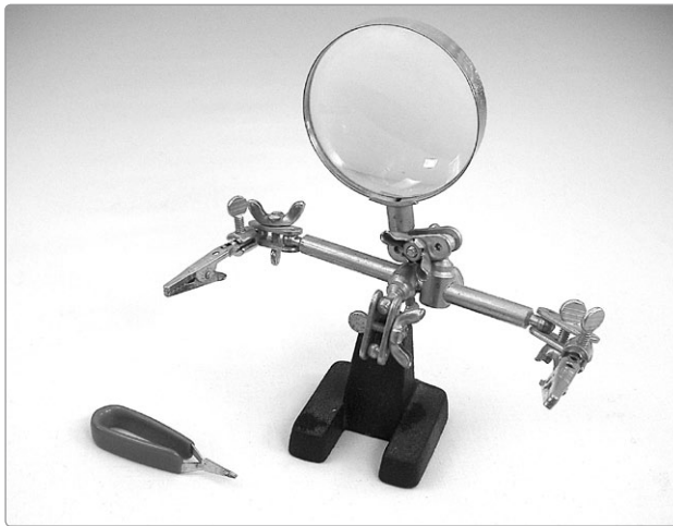
FIGURE A-17: A heat sink (left) and helping hands (right)
