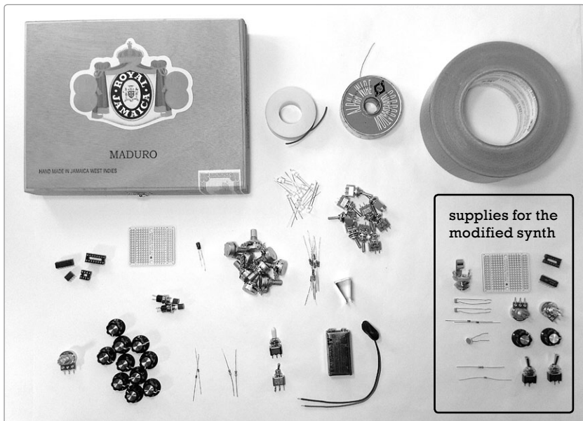
FIGURE 16-2: Tools and supplies; the parts for the modified Single-Chip Space Invader Synth are clustered in the lower-right corner of the bottom image (not shown: amp, instrument cable, hacksaw, marker, and multimeter)
