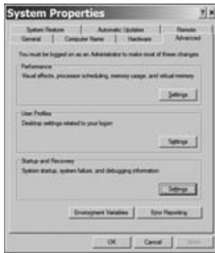
Figure 4-3: Click the Settings button in the Startup And Recovery box to turn off automatic recovery.
