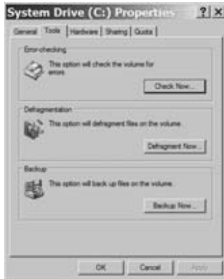
Figure 20-3: Use the Properties window for each drive to defragment that drive.
