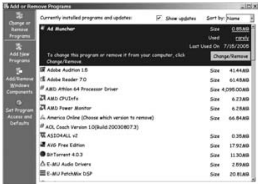
Figure 10-1: Use the Add Or Remove Programs tool to delete a damaged program.
