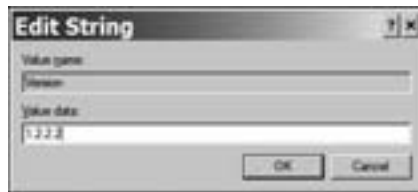
Figure 9-5: Use the Edit String dialog box to change the value of a Registry key.
