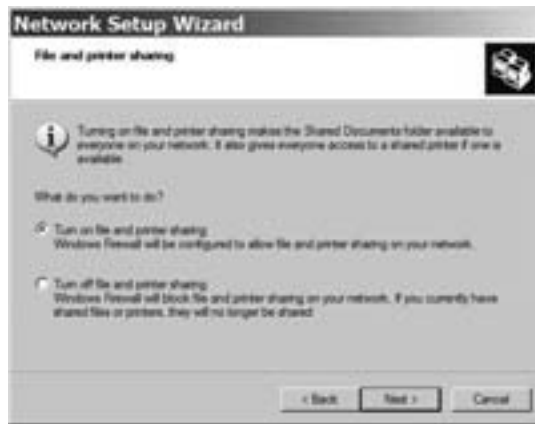
Figure 14-2: Use the Network Setup Wizard to turn on file sharing.
