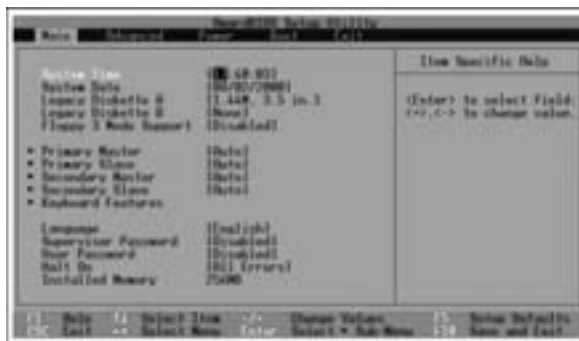
Figure 16-6: The BIOS Setup Utility might show the hard drive configuration options as primary and secondary masters and slaves . . .
