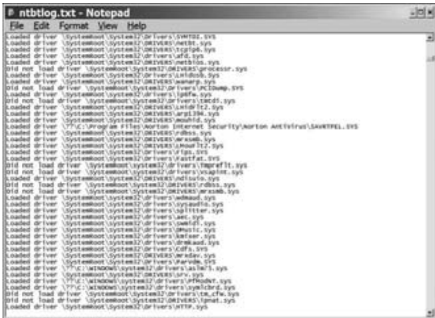
Figure 3-5: The Boot Log includes a status line for each driver that loads with Windows.
