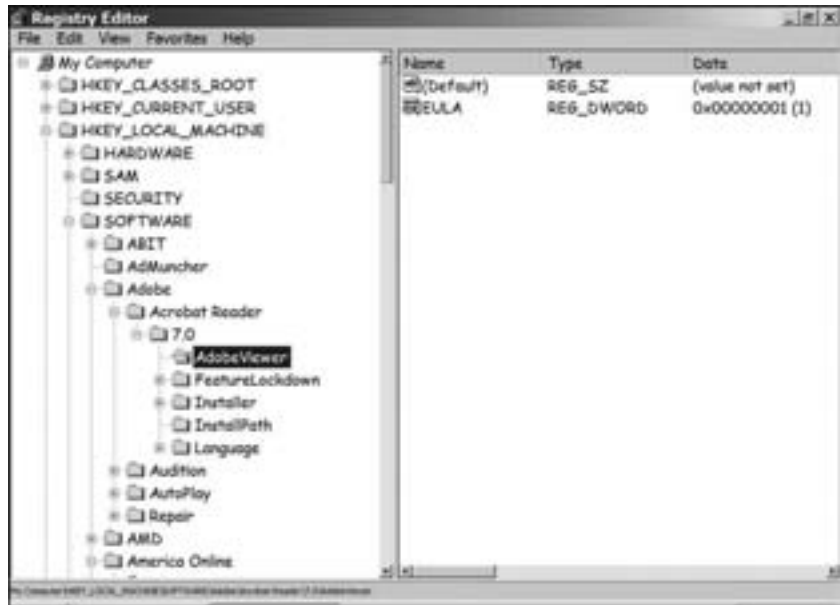
Figure 9-3: Many Registry items are nested several layers into the tree structure.
