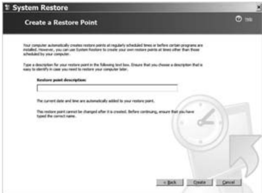
Figure 7-3: The Create A Restore Point window includes space for a description of the new restore point.
