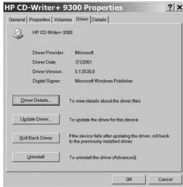
Figure 7-1: Use Roll Back Driver to return to an earlier version of a device driver.
