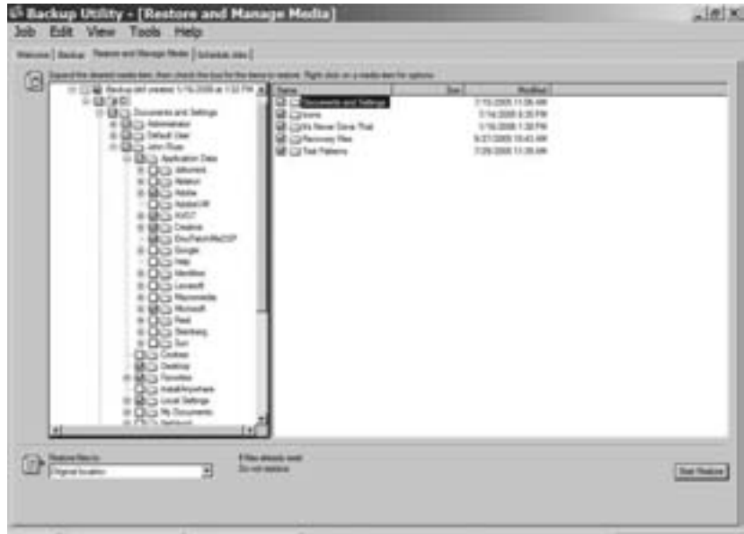
Figure 20-2: Use the Restore And Manage Media tab to recover files and folders from your backup.
