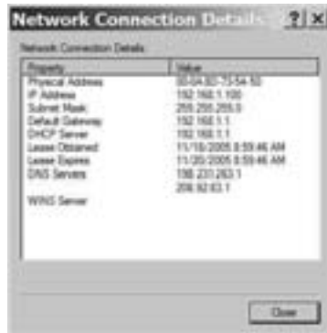
Figure 19-3: Make a written copy of the Network Connection Details before you reinstall Windows.
