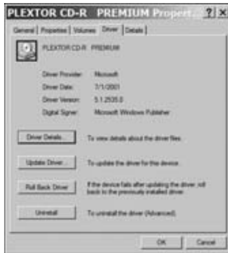
Figure 5-6: Use Roll Back Driver to return to an earlier version of a device driver.
