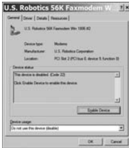
Figure 5-3: The Device Manager links to Properties windows that identify driver problems.
