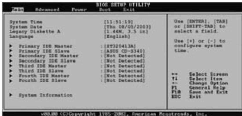
Figure 8-1: This AMIBIOS utility shows the IDE drive settings on the Main menu . . .
