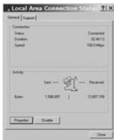
Figure 12-2: The Connection Status window shows the current condition of a network connection.
