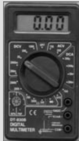
Figure 1-4: Set the meter to one of the DC V ranges.
