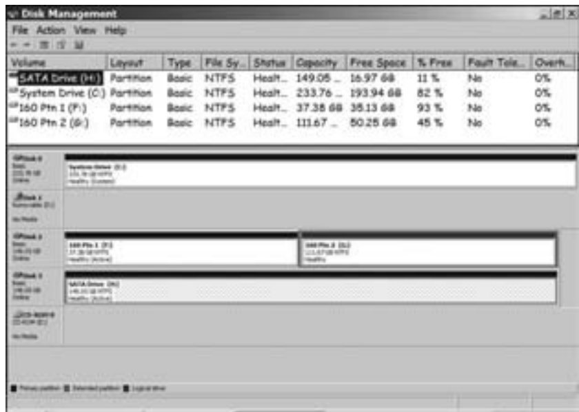
Figure 19-4: Use the Disk Management program to format a nonsystem drive
