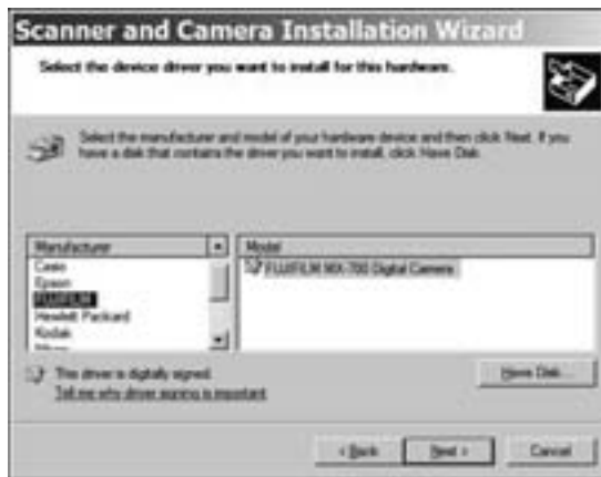
Figure 5-4: Use the Have Disk button to install a device driver from a file.
