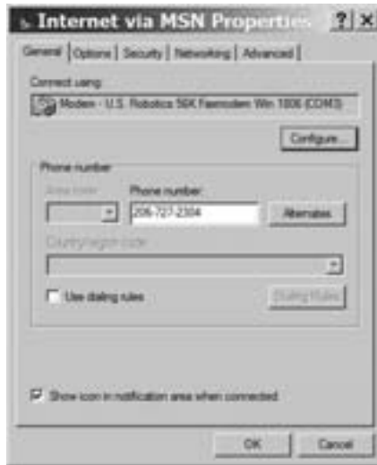
Figure 13-7: Use the dial-up networking Properties window to set the ISP's telephone number.
