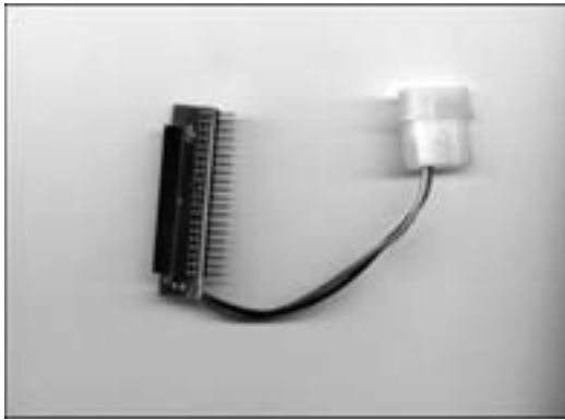
Figure 16-5: Using a 2.5-inch hard drive with a standard IDE cable requires a special adapter.
