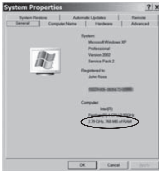
Figure 17-1: The speed of the CPU and the amount of memory available to Windows appears at the bottom of the list of system details.
