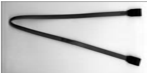
Figure 16-2: SATA data cables are smaller and easier to handle than IDE cables.
