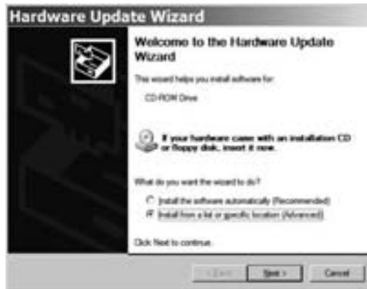
Figure A-1: To solve a Code 31 error, run the Hardware Update Wizard.
