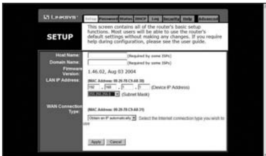
Figure 13-8: This Linksys router configuration utility specifies the IP addresses that the router uses to connect to both the Internet and the local network.
