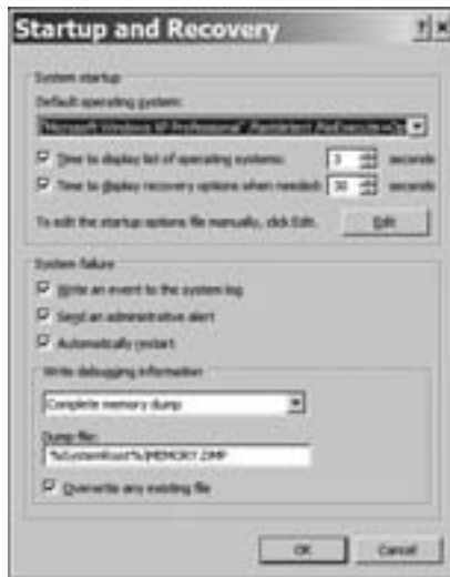
Figure 4-4: The Automatically Restart option is located in the System Failure section of the Startup And Recovery window.
