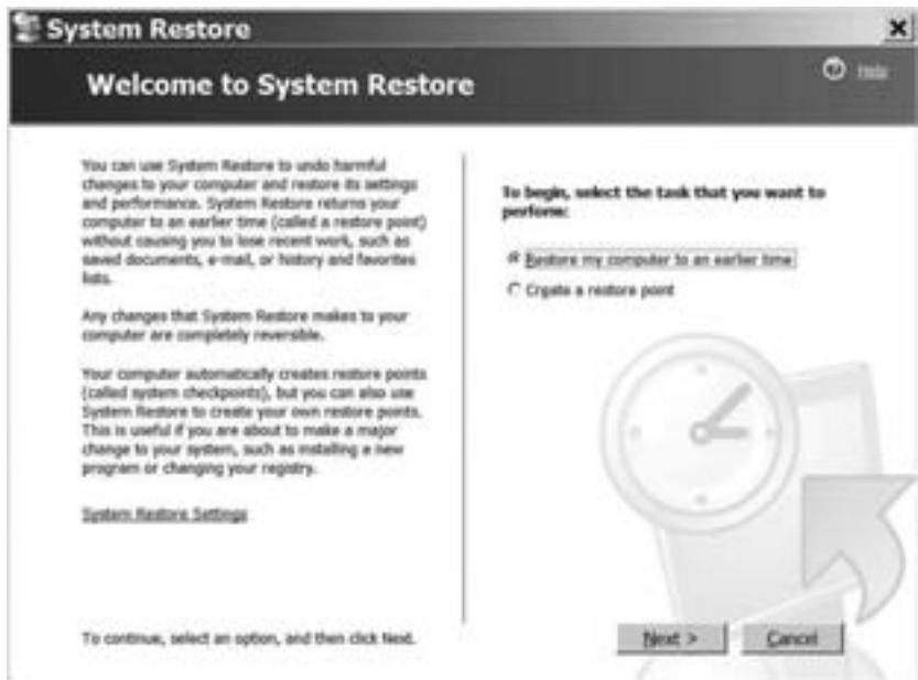
Figure 7-2: Use the System Restore tool to create a new restore point or to return to an earlier configuration.
