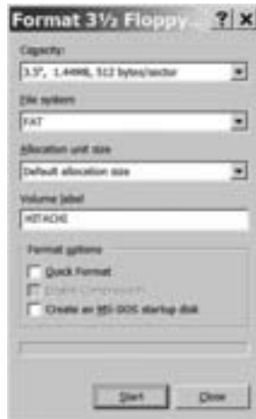
Figure 20-5: Use the Format tool to create an MS-DOS Startup Disk.
