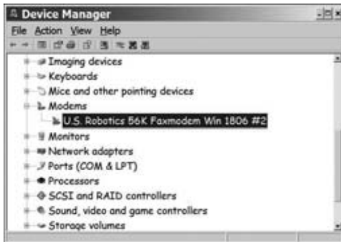
Figure 5-2: The Device Manager has identified a problem with the modem driver.
