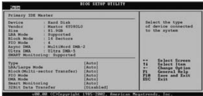
Figure 8-3: The BIOS tool includes settings for all the essential IDE device values.
