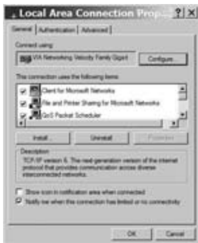
Figure 14-1: The Local Area Properties window controls the network configuration.
