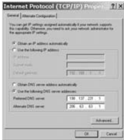
Figure 13-1: In this example, the network automatically assigns an IP address.
