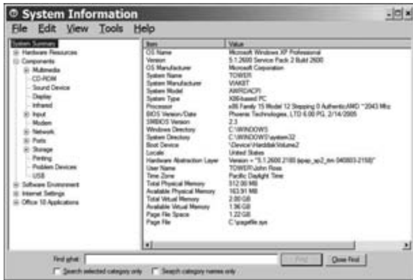
Figure 1-6: Use the System Information tool to identify the BIOS version and date.
