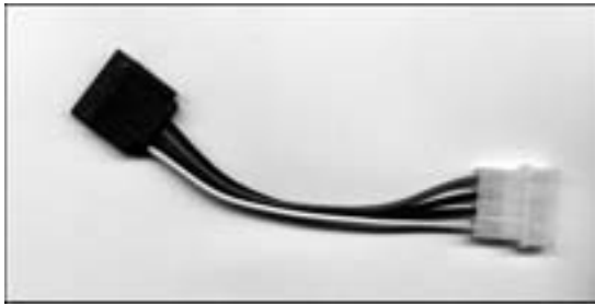
Figure 16-3: Use a power adapter to connect an SATA drive to an older power supply.
