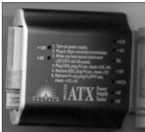
Figure 1-3: A simple power supply tester makes it easy to check power supply voltages.
