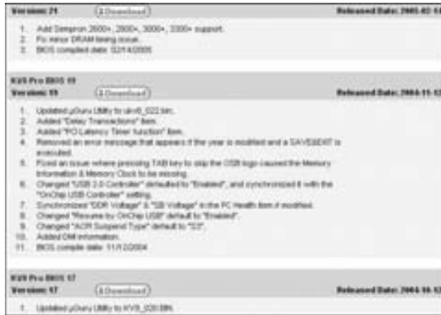
Figure 11-2: In this example, you must update to version 21 to use the motherboard with AMD Sempron processors.
