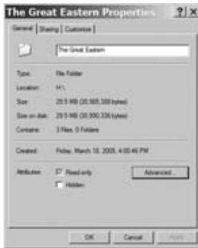
Figure 14-5: To change the Read-only status of a file or folder, open the Properties window.
