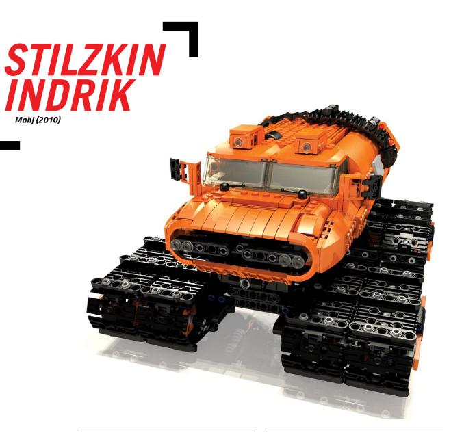
This model of a fictional arctic exploration vehicle features four tracks driven by two independent motors and steered by slewing, as well as powerful lights for nighttime operations. It's not fast, but it climbs through deep snow and pulls two fully loaded cargo sledges without any difficulty.
