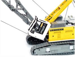
This model of a Liebherr dragline excavator is split into two independent parts. The chassis has its own power supply and IR receiver, which means the superstructure can make an unlimited number of rotations, because not a single wire connects it to the chassis.
