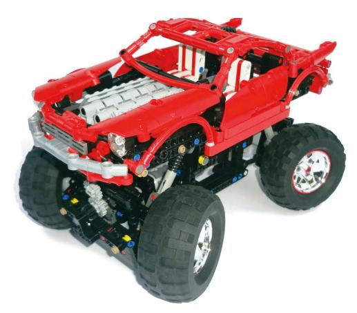
This small-scale model of a monster truck combines impressive functionality with a sleek body that can be removed. The chassis features an independent suspension with floating axles, a 4×4 drive with a central differential, all-wheel steering, and a V8 piston engine, which is massive at this scale. The body is skillfully shaped with just a handful of small panels and axles, the doors can be opened, and the rims are custom chromed.
