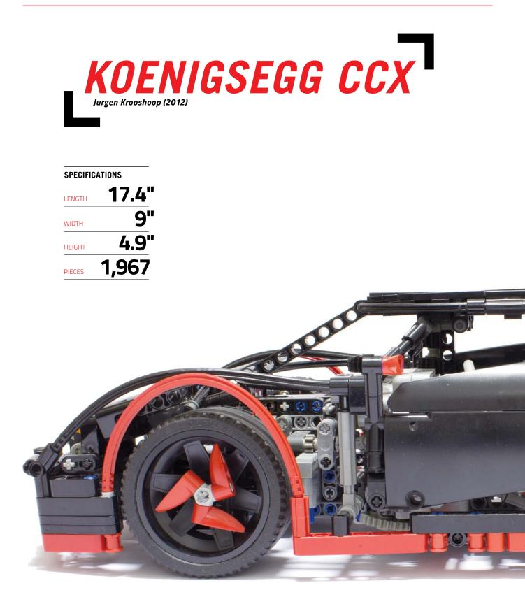
This model of the exotic Swedish supercar is packed with features. Among them are a fully independent suspension, positive caster and camber angles on the front axle, a hand-of-God steering system with a working steering wheel and Ackermann geometry, a V8 piston engine, a six-speed transmission, and an opening hood and trunk. Most notably, the model reproduces the trademark Koenisegg doors, which move outward and rotate at the same time.
