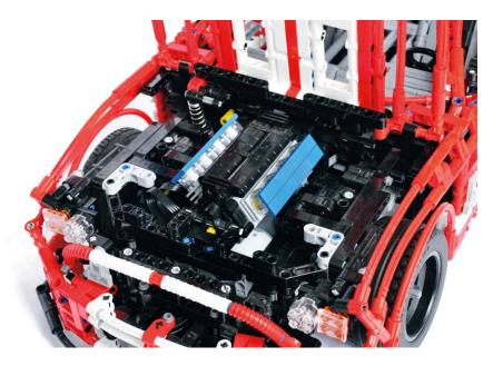
This 1:8 scale model of the Ford Mustang Shelby GT500 comes with a McPherson front suspension and live axle in the rear, as well as working disc brakes on all wheels, with a moving brake pedal inside the cabin. Front wheels have positive camber, with a caster and kingpin angle, and are steered with Ackermann geometry. The sequential 5+R transmission features an automated clutch, the hood opens to reveal a V8 piston engine, the trunk can be opened, and the doors even have locks!
