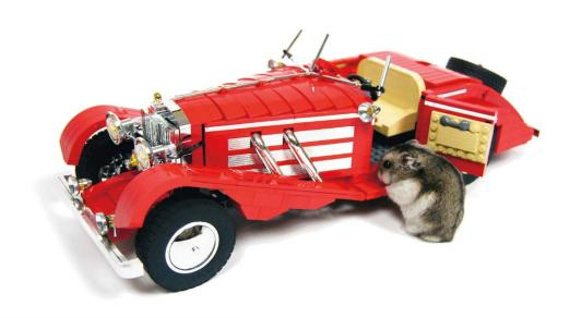
This is a relatively simple model, combining a brick-built chassis with two Power Functions motors—a PF L motor for driving and a Servo motor for steering. The detailed body consists of more than 1,000 LEGO pieces, but there's no suspension system, and the technical sophistication ends with a working steering wheel. The resulting model includes just 8 gear wheels but has more than 80 curved slopes as well as a few custom-chromed pieces.
