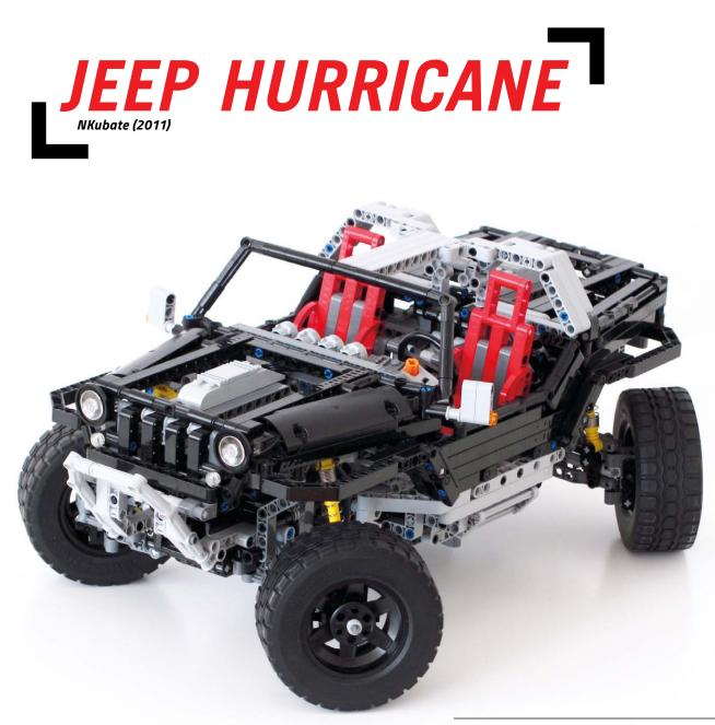
This model attempts to re-create the advanced functions of a Jeep concept vehicle. It includes a fully independent suspension, all-wheel drive, two V8 piston engines, a drivetrain that allows normal drive or skid steering, and two steering modes (regular and "toe-in" steering). The completed model includes approximately 60 gear wheels and is built so densely that it weighs 4.4 lb (2 kg), despite being rather compact.
