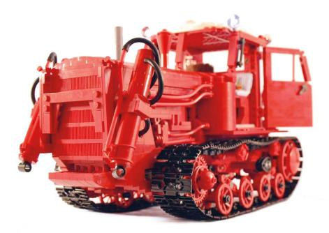
You start the DT-75 tractor via a recoil starter, just like a lawn mower. The starter activates a small combustion engine, which then starts the huge diesel engine that powers the tracks.
