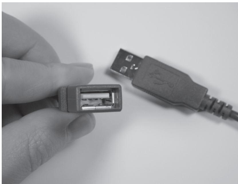
Figure 4-2: USB type A female connector.
