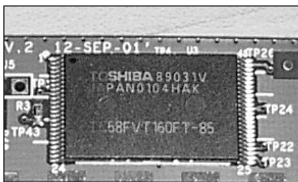
Figure 5-6: 2MB nonvolatile RAM (flash memory)
