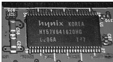
Figure 5-5: 8MB dynamic random access memory (DRAM) module
