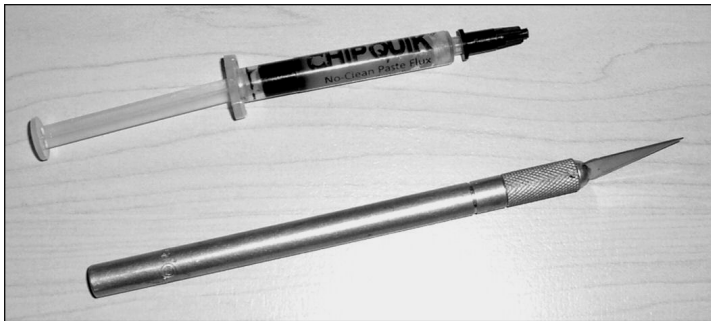
Figure 8-2: A tube of Chip Quik (top) and an X-ACTO knife (bottom)
