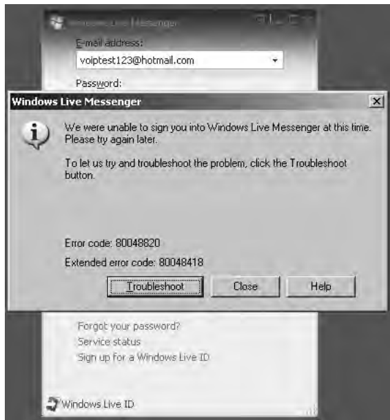
Figure 8-20: Failed SSL man-in-the-middle attack under Live Messenger
