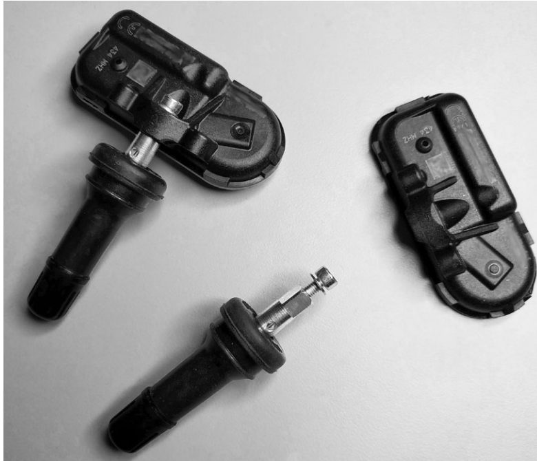
Figure 12-3: Two TPMS sensors
