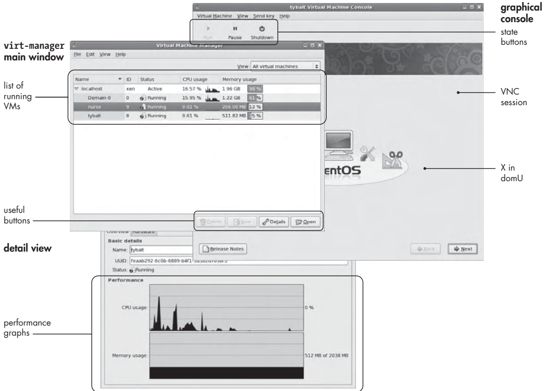
Figure 6-1: Here you can see the virt-manager UI. It has a main screen that lists virtual machines; a detail view that shows VM resources, performance, and statistics; and a framebuffer console as well as a text console interface.
