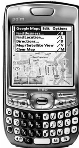
Figure 14-3: The Palm Treo 680 smartphone uses the Palm OS operating system.
