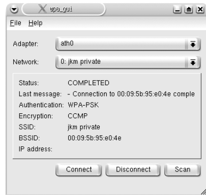
Figure 7-6: wpa_supplicant's GUI provides WPA client support ( http://hostap.epitest.fi/wpa_supplicant/ ).
