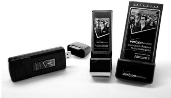
Figure 13-2: Broadband network adapters are available as USB, ExpressCard, and PC Card.
