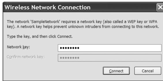
Figure 5-11: When the Wi-Fi control program detects an encrypted network, it will ask for the network key.
