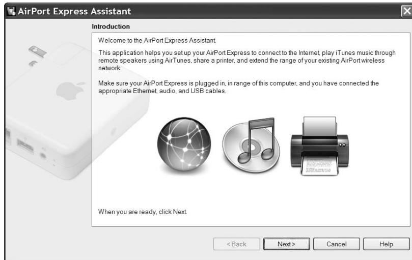
Figure 8-4: The AirPort Express Assistant for Windows provides a step-by-step process for setting up an AirPort Extreme network.
