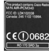
Figure 17-3: Every wireless adapter has a unique FCC ID number.
