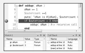
This screenshot shows the recursion program being debugged visually in the IDE Ruby In Steel. I can step through the source code, use the call stack to keep track of the current "level" of recursion (how many times the addup method has been called), and use the Watch window to monitor the current values of the variables.
