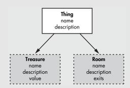
This diagram shows a Thing class that has a *name* and a *description* (in a Ruby program, these might be internal variables such as @name and @description plus some methods to access them). The Treasure and Room classes both descend from the Thing class, so they automatically "inherit" a *name* and a *description*. The Treasure class adds one new item, *value*, so it now has *name*, *description*, and *value*. The Room class adds *exits*—so it has *name*, *description*, and *exits*.
