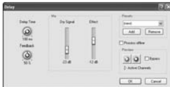
Figure 4-17: The Delay dialog box lets you define a delay time and feedback to create an echo within an audio file.
