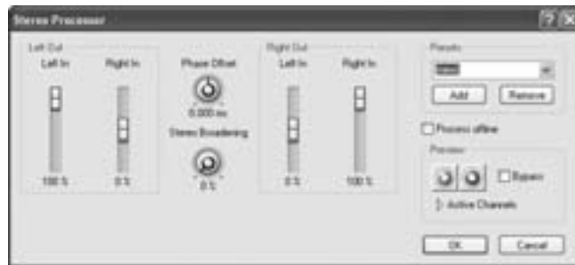
Figure 4-13: The Stereo Processor dialog box lets you adjust the stereo sound of an audio file.
