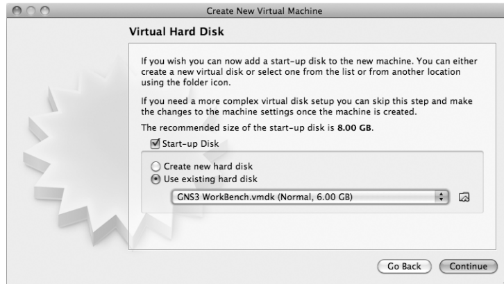
Figure 2-6: Selecting the VMware Disk Image to use with VirtualBox
