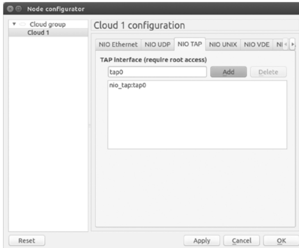
Figure 10-5: Configuring NIO TAP with tap0 on Ubuntu Linux
