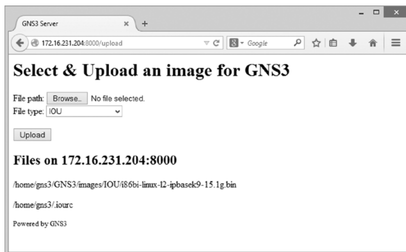
Figure 9-11: Select and upload your IOU image files.
