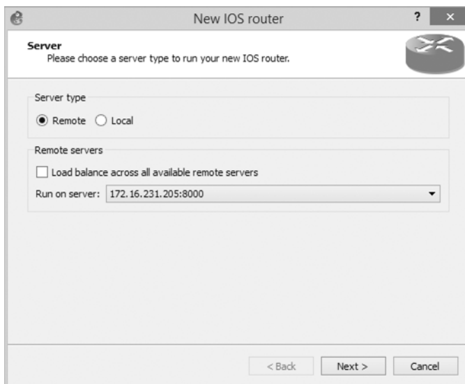
Figure 10-15: Selecting the Remote server type
