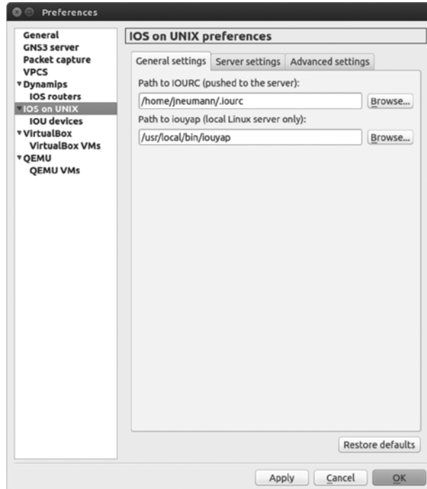
Figure 9-1: IOS on UNIX preferences, General settings tab
