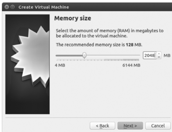
Figure 6-21: Adjust the memory size.
