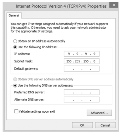
Figure 10-2: Configuring your Loopback Adapter driver with an IP address
